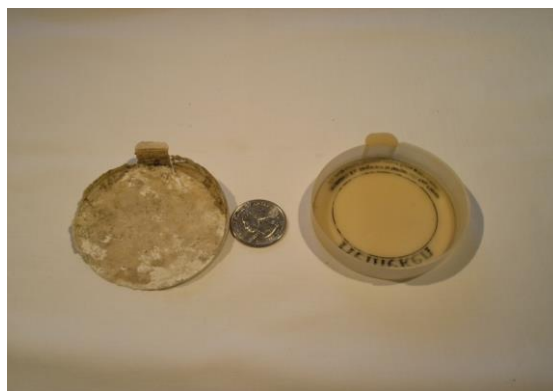
Figure 3: Biodegradation of PHA Lid Material in Seawater after 3 Months of Immersion.
