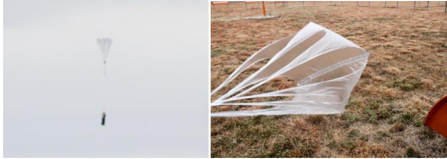
Figure 2: Decelerator in Flight (left) and Ground Wind Inflation (right).
