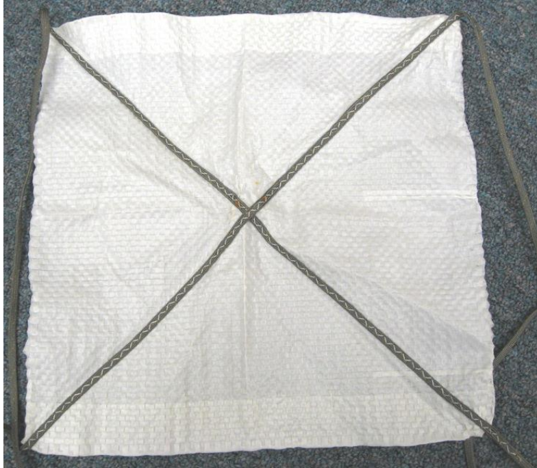
Figure 16: Post Test Photograph of Top Surface of Square Decelerator.
