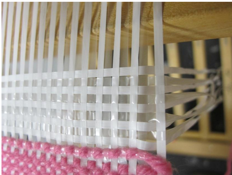
Figure 8: Details of PVOH/PHA Weave In-Process.
