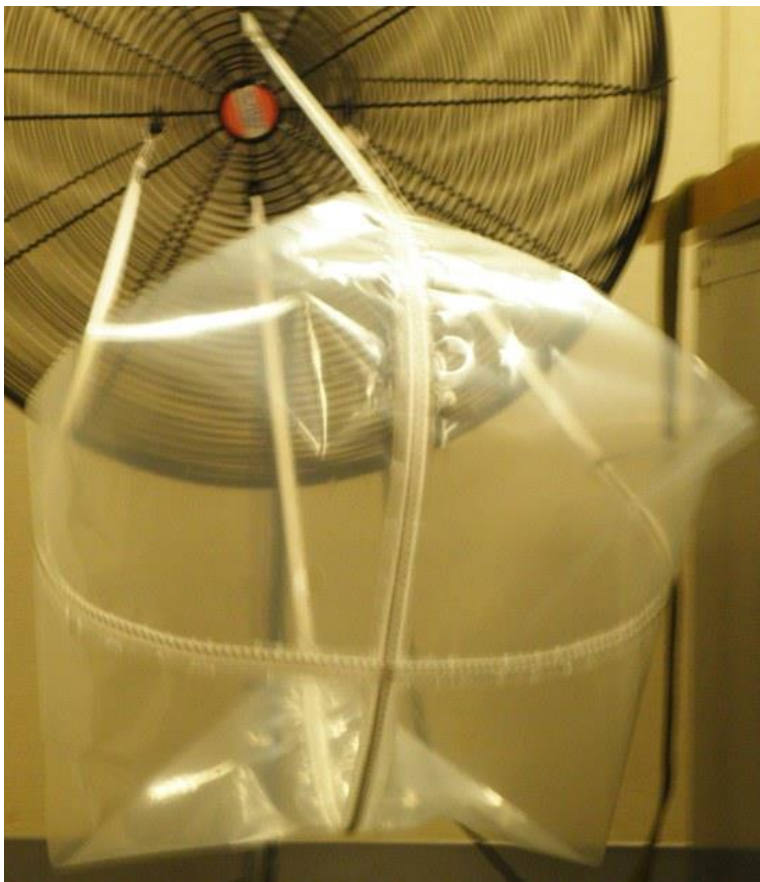
Figure 14: Simple Inflation Test of Prototype PHA Decelerator.
