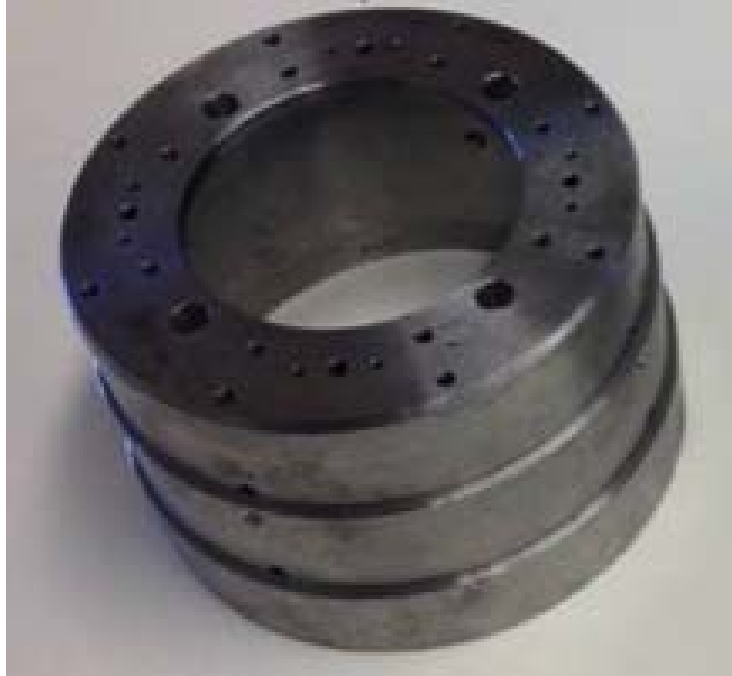
Figure 7. Stator Support Structure. Source: [5].
