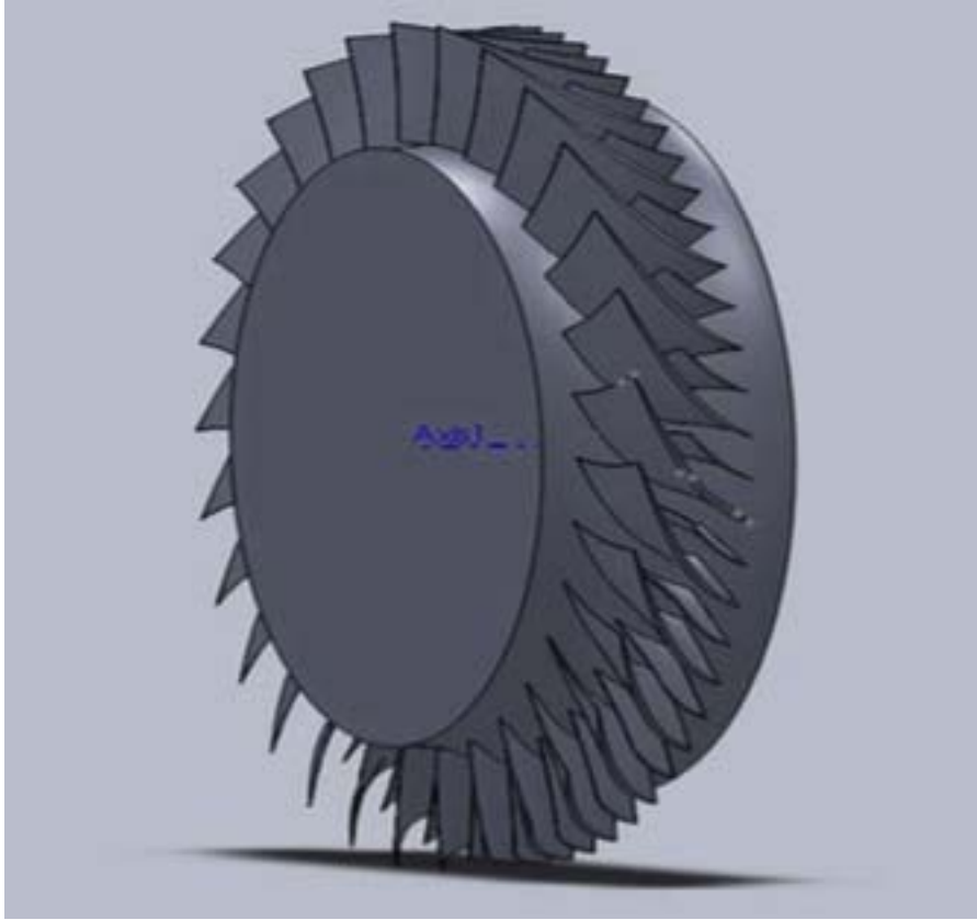
Figure 2. Wennerstrom's Supersonic Axial Rotor with Splitter Vanes. Source: [4].
