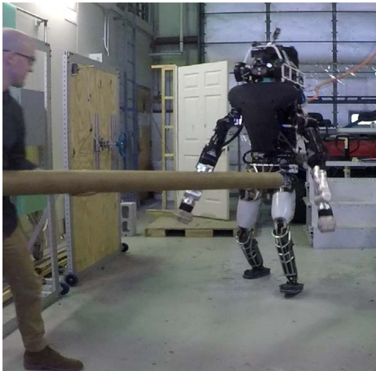
Figure 2 - Demonstration of the robot's dynamic balancing
