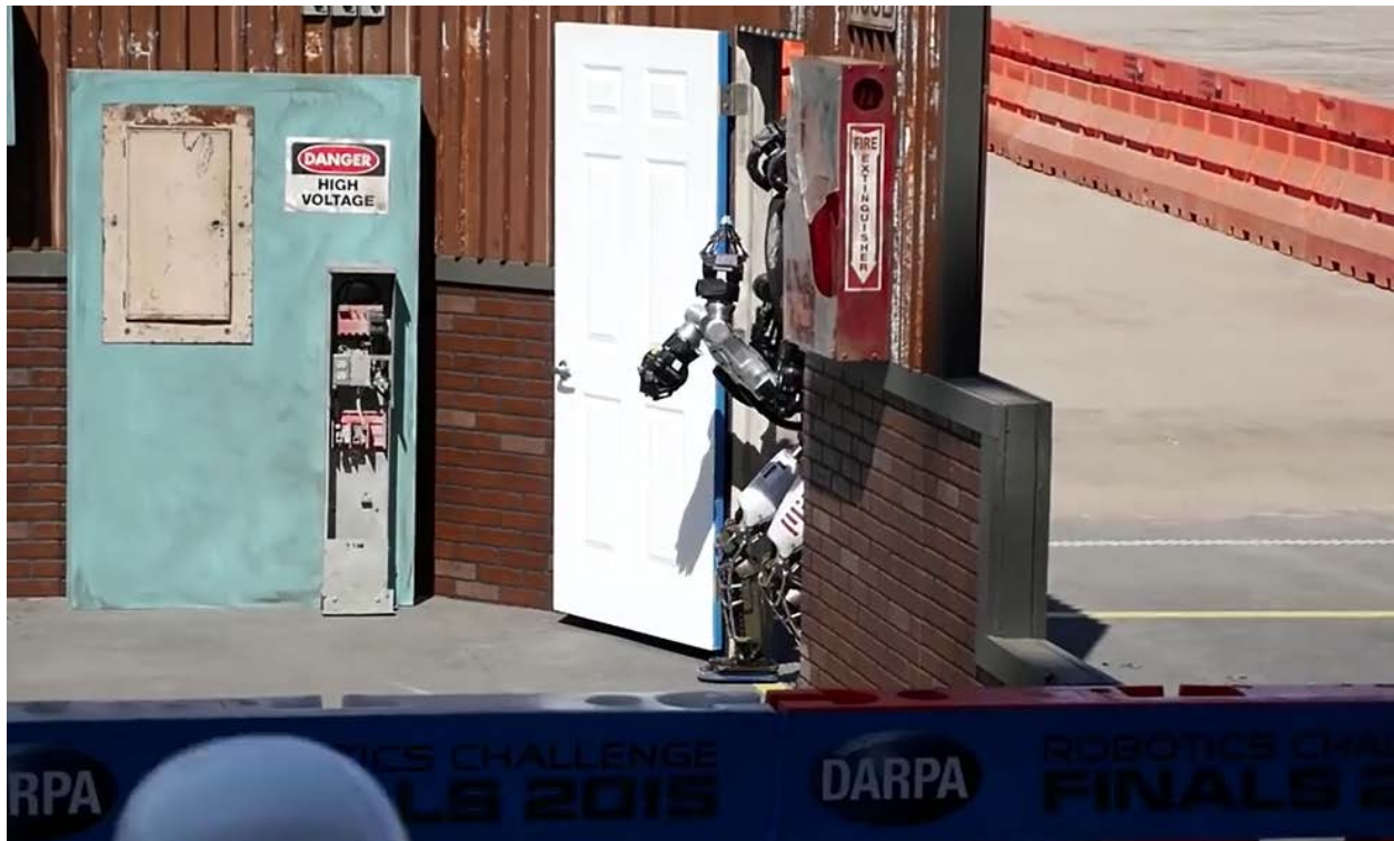
Figure 8 - Atlas Robot successfully opening a door and crossing the threshold.
