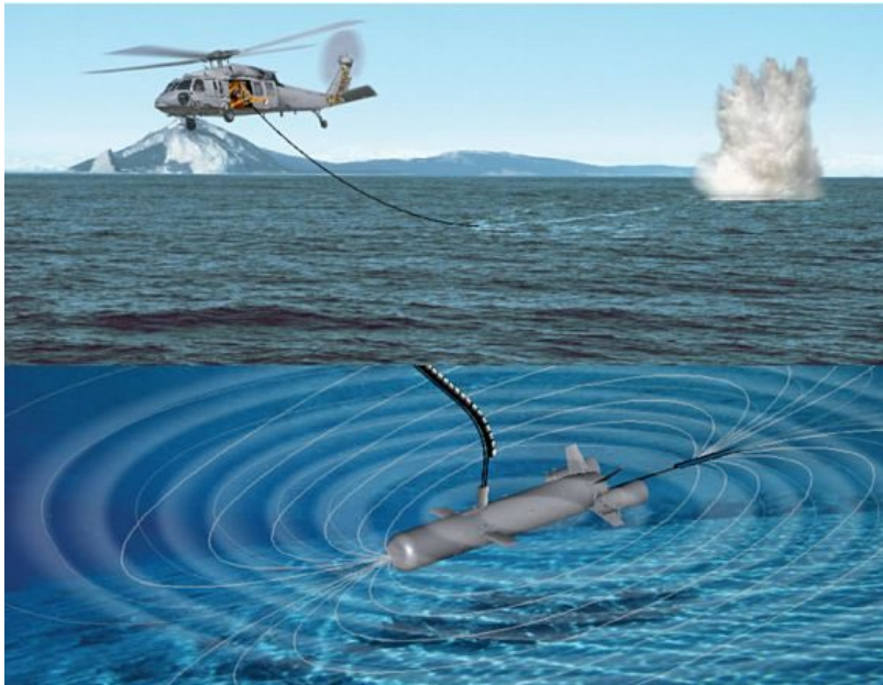
Figure 18. Depiction of an AMNS Barracuda Launched from Helicopter. Source: PennWell Corporation (2014)
