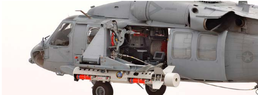
Figure 11. MH-60S Helicopter Equipped with AN/AQS-235 AMNS. Source: Mine Warfare Assn. (2013)
