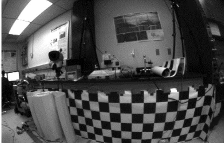
Fig. 14 Camera scene ( 376 \times 240 pixel image): DC light source is not in the FOV of the camera, which is moving along the x-direction
