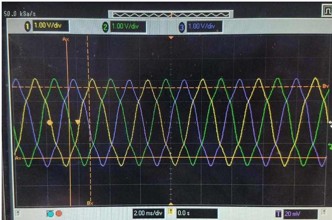
Figure 11. AC Waveforms from Poseidon RC Boat Motor
