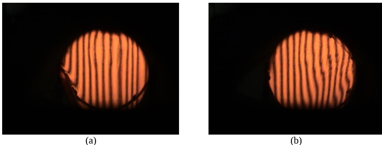
Figure 5. Line deviation and shear patterns: Images showing (a) an example of a line deviation for an amber tinted protective mask outsert and (b) an example of a shear pattern.
