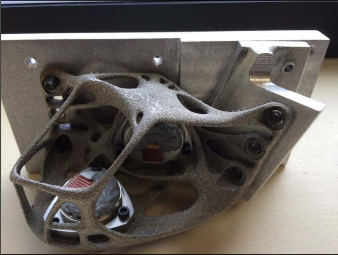
Figure 2. Accelerometer Bracket Designed Using Topology Optimization and Fabricated Using Direct Metal Laser Sintering Technology
