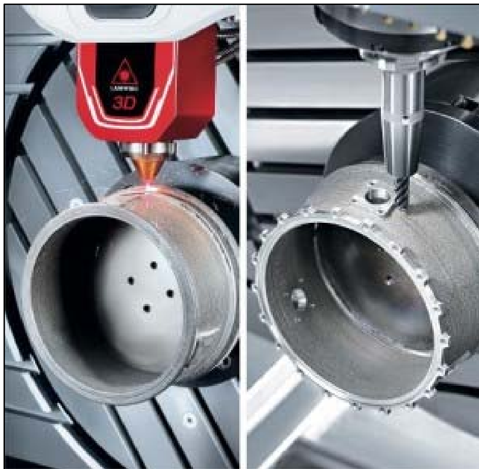
Figure 4. DMG Mori Lasertec System Depositing Metal Powder Onto Part [3]
