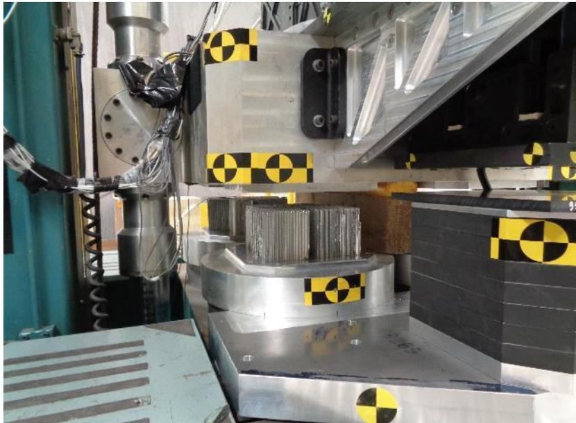
**Figure 13. Carriage Programmer (Hexcel) Used for Test Series 4**
