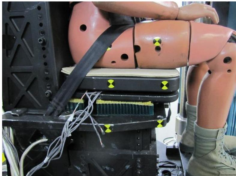
**Figure 11. Seat Pan Programmer (Stimulite TPE) Used for Test Series 2**
