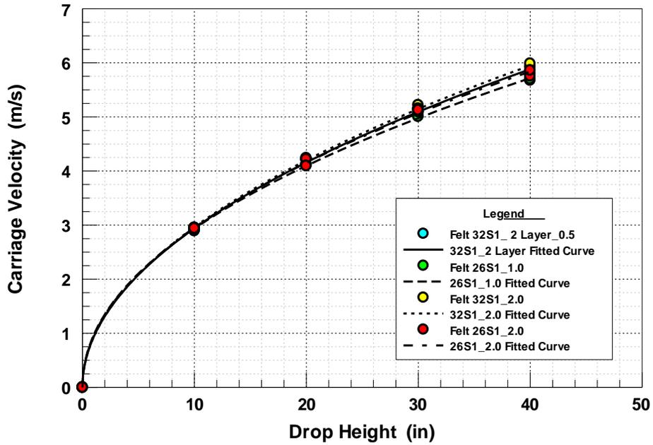
Figure 20. Peak Carriage Velocity as a Function of Drop Height for Test Series 1 (WS2)
