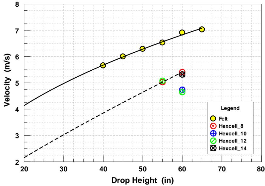
Figure 32. Peak Seat Pan Velocity as a Function of Drop Height: Test Series 4 (WS3)
