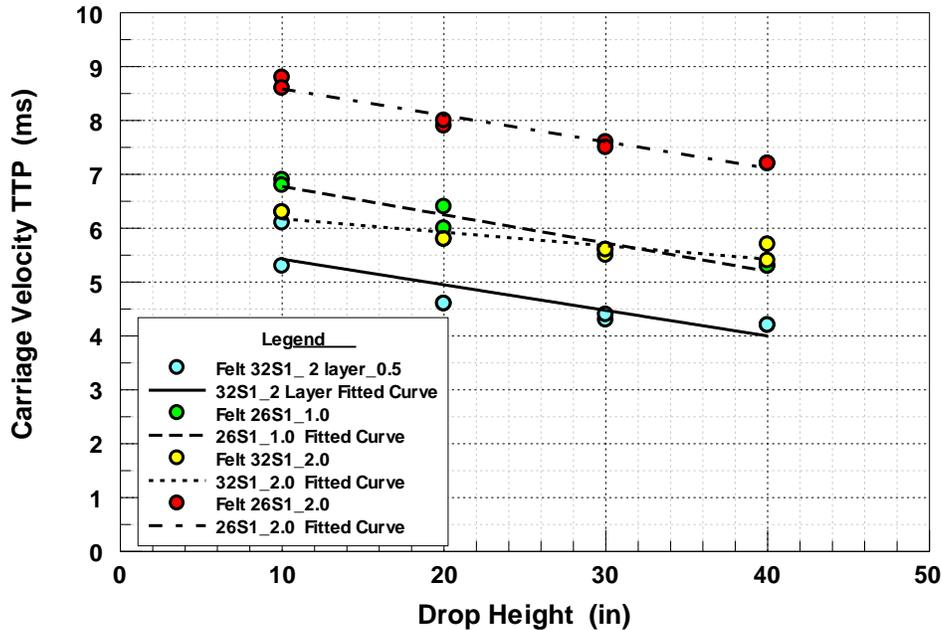
Figure 21. Carriage Velocity TTP as a Function of Drop Height for Test Series 1 (WS2)
