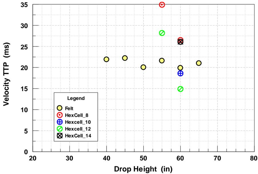
Figure 33. Seat Pan Velocity TTP as a Function of Drop Height: Test Series 4 (WS3)
