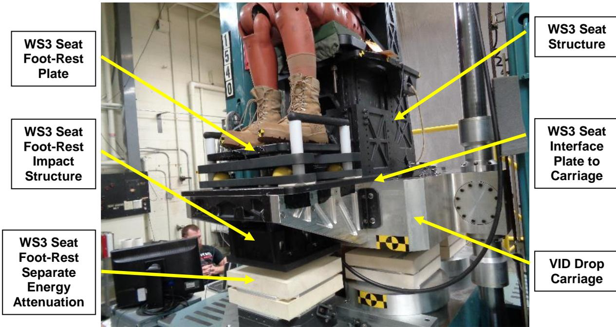
**Figure 9. Foot-Rest Impact Structure for WS3 Seat**
