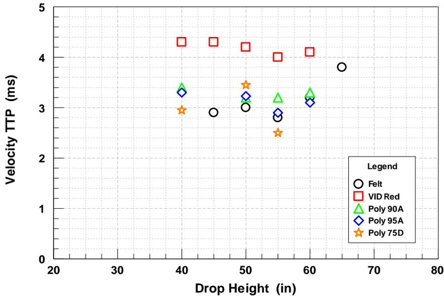
Figure 31. Foot Rest Velocity TTP as a Function of Drop Height: Test Series 4 (WS3)
