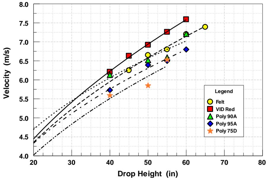
Figure 30. Peak Foot Rest Velocity as a Function of Drop Height: Test Series 4 (WS3)
