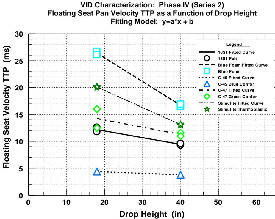
**Figure 29. Floating Seat Velocity TTP as a Function of Drop Height:Test Series 2 (WS2ms)**
