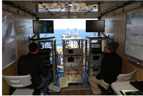
(b) Transmit and system timing hardware are in the far right rack; receiver, signal analysis, and power hardware are in the center; data acquisition hardware is at left.
