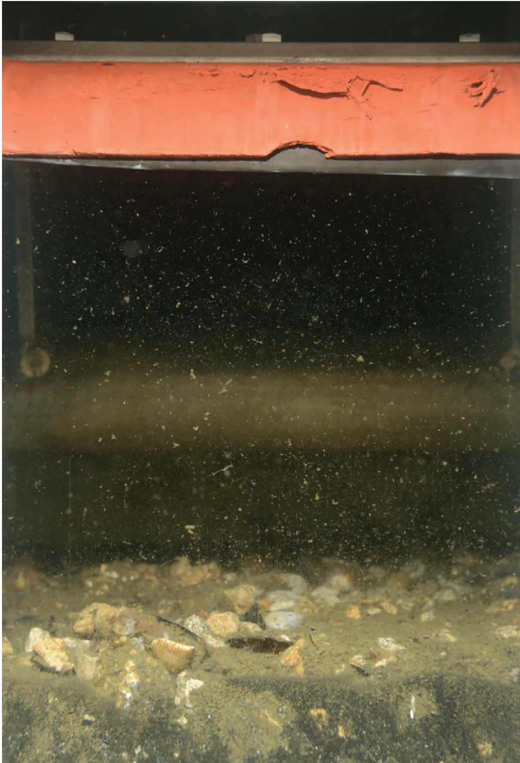
Figure 7: This profile image from Station 5-3 shows surface armoring from the pebbles used as a carrier vehicle for the activated carbon in the AquaGate amendment that was placed under and around Pier 7. Scale: width of profile image = 14.5 cm.
