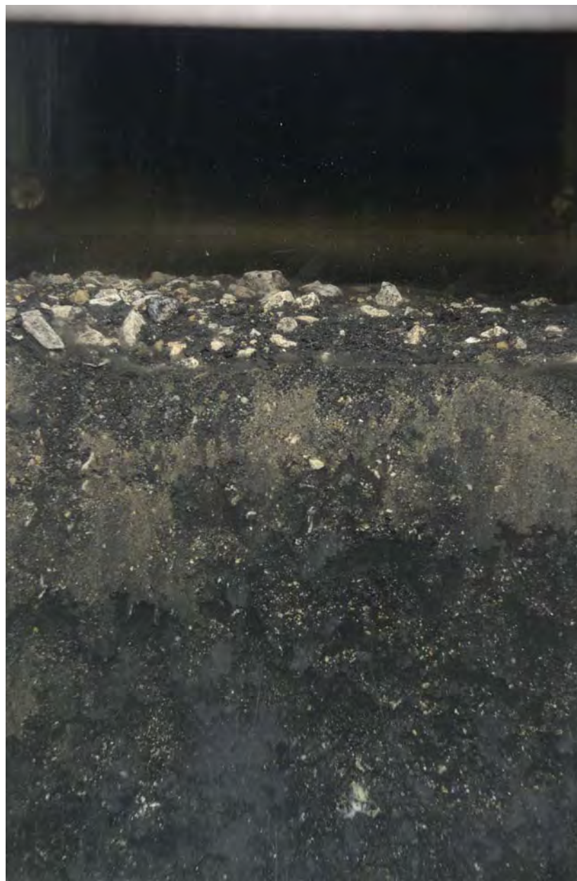
Figure 14: These profile images from Stations 3-4 (left) and 5-4 (right) show how the activated carbon covering on the carrier particles for the AquaGate+PAC™ has dissolved off the carrier granules, leaving a surface armoring of white pebbles while the carbon particles are being re-worked throughout the underlying sediment column. Scale: width of each image = 14.5 cm.
