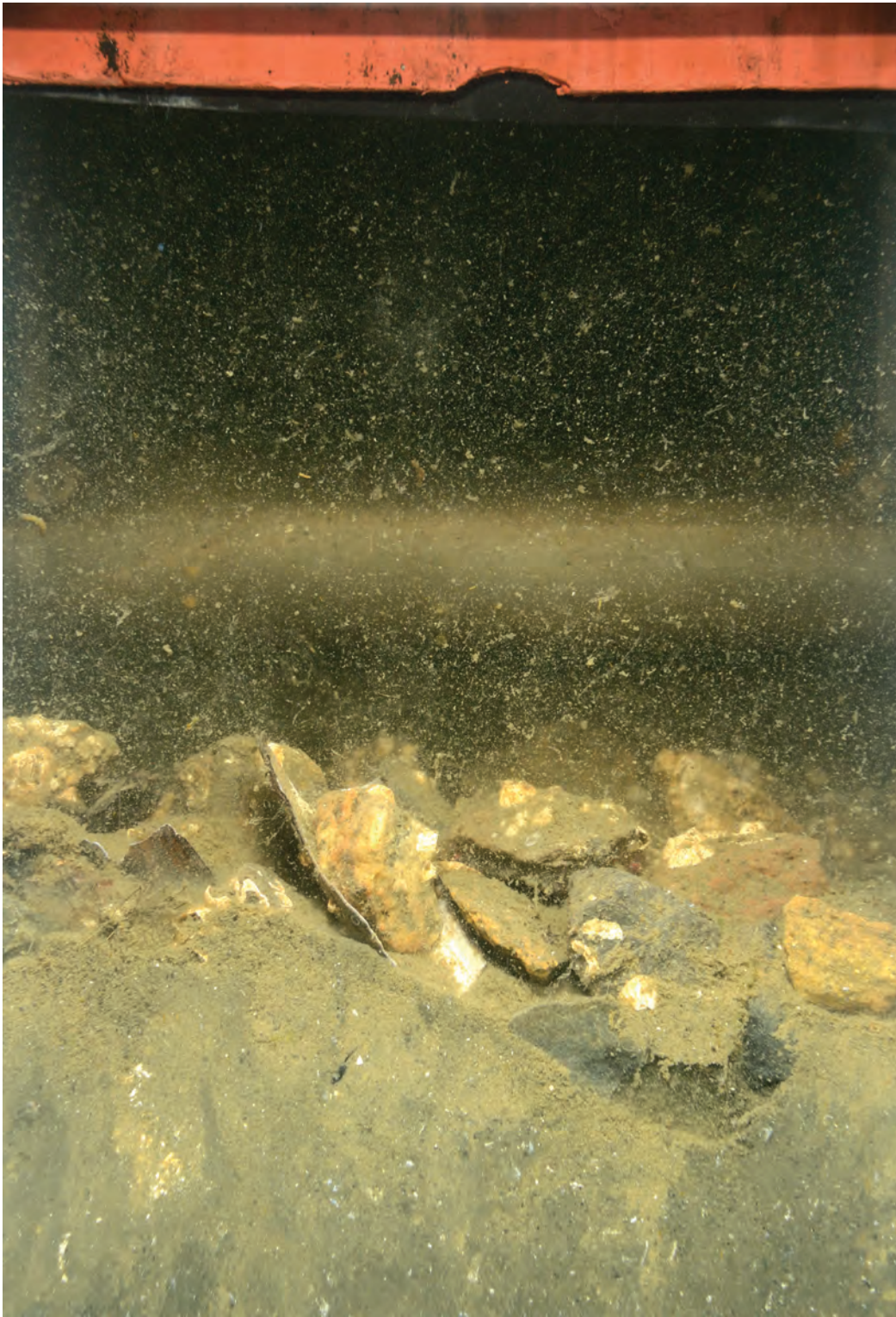
Figure 6: As in past surveys, the SPI photos from Station 1-3 show an armor layering of pebble and cobbles over silty very fine sand. Scale: width of profile image = 14.5 cm.
