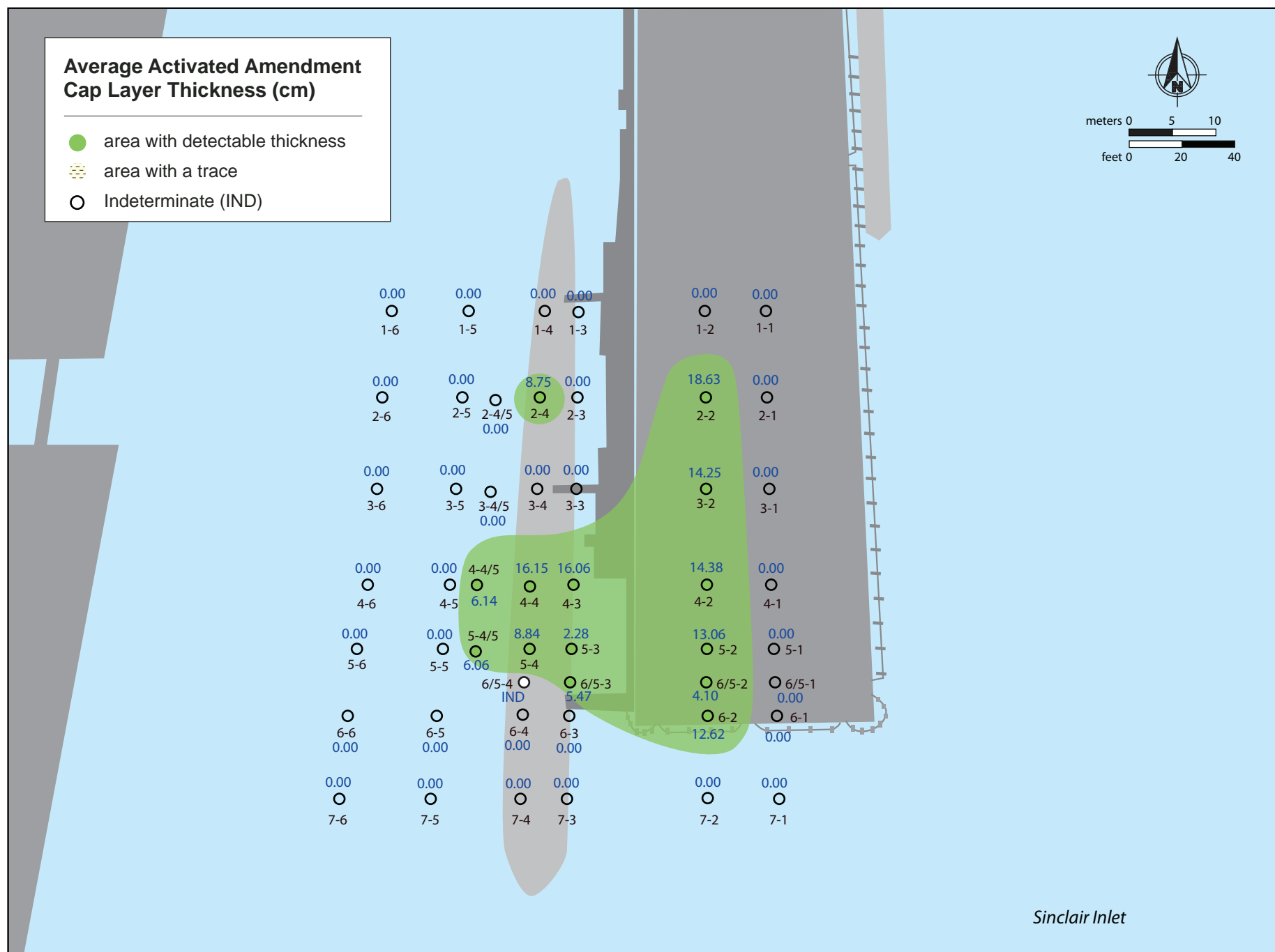
Figure 9: Spatial distribution and mean depositional thickness (cm) of the AquaGate +PAC™ material placed at locations in and around Pier 7 at the PSNS & IMF Bremerton site.
