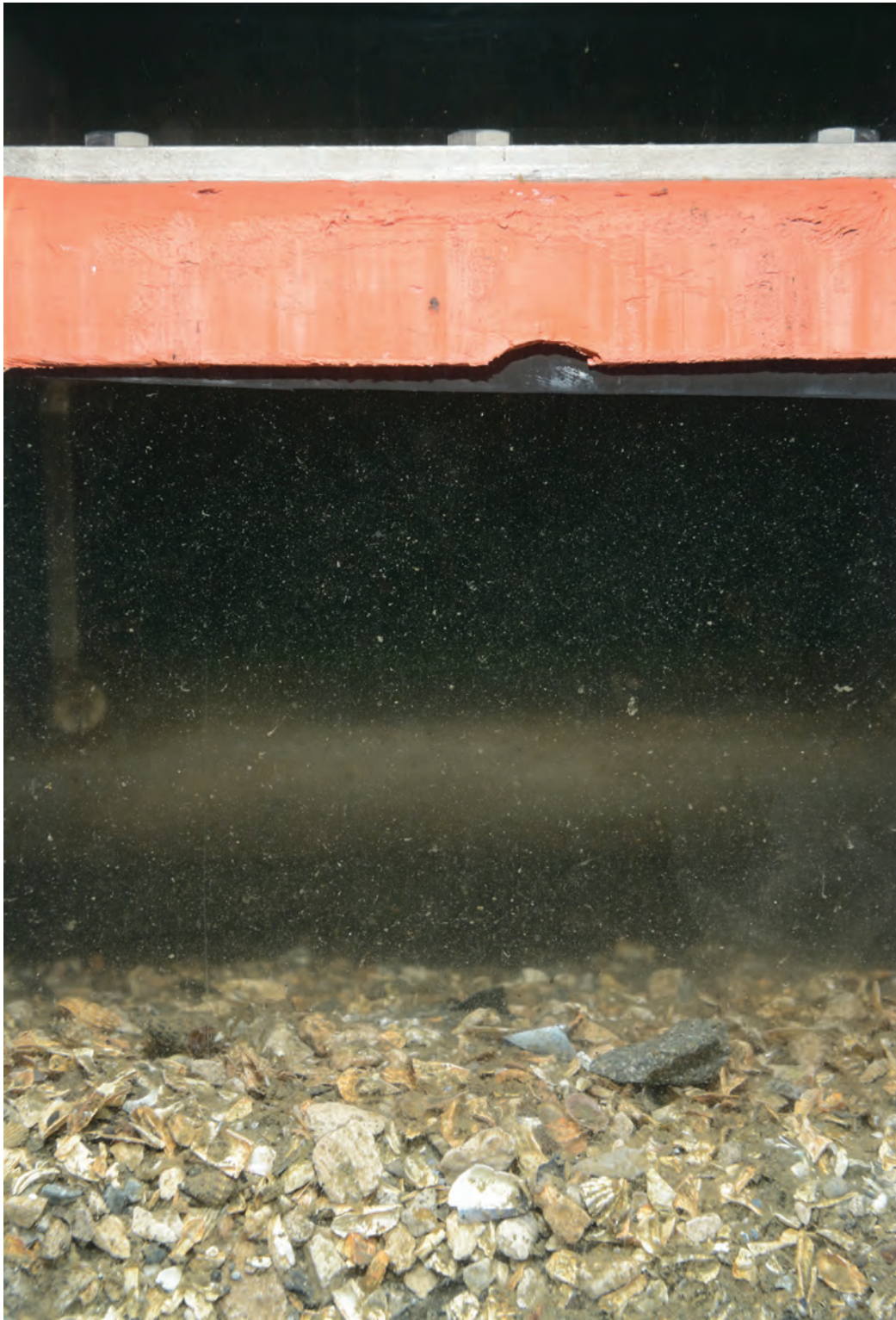
Figure 7: This profile image from Station 2-3 shows surface armoring from the pebbles used as a carrier vehicle for the activated carbon in the AquaGate amendment that was placed under and around Pier 7. Scale: width of profile image = 14.6 cm.
