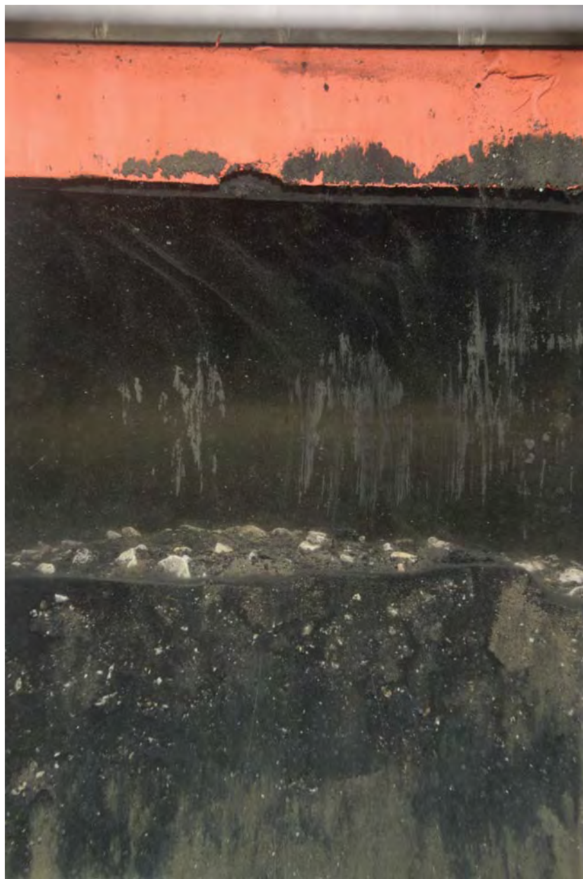
Figure 14: These profile images from Stations 3-4 (left) and 5-4 (right) show how the activated carbon covering on the carrier particles for the AquaGate+PAC™ has dissolved off the carrier granules, leaving a surface armoring of white pebbles while the carbon particles are being re-worked throughout the underlying sediment column. Scale: width of each image = 14.5 cm.
