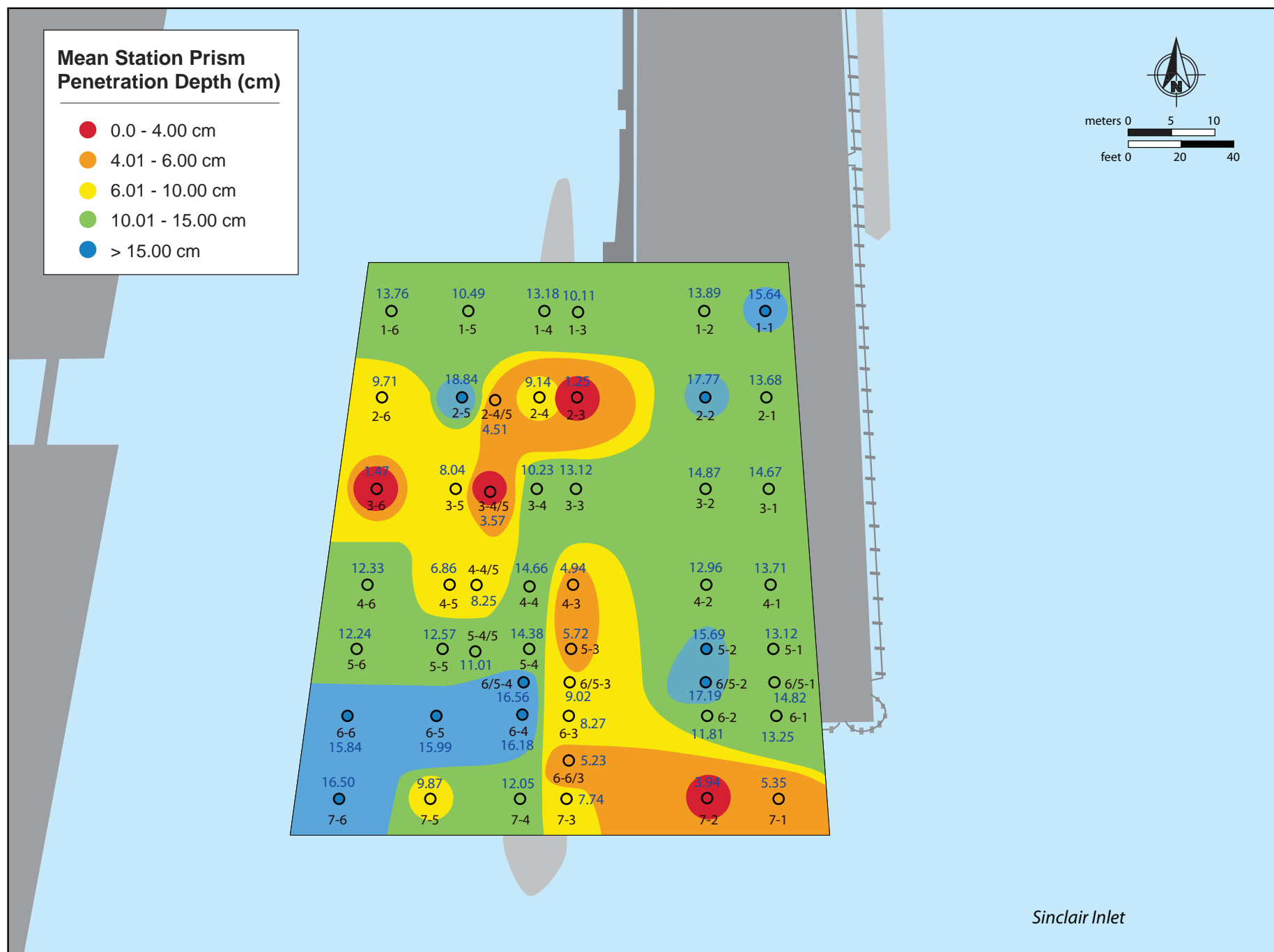
Figure 8: Spatial distribution of mean camera prism penetration depth (cm) at Pier 7 at the PSNS & IMF Bremerton site in July 2015.
