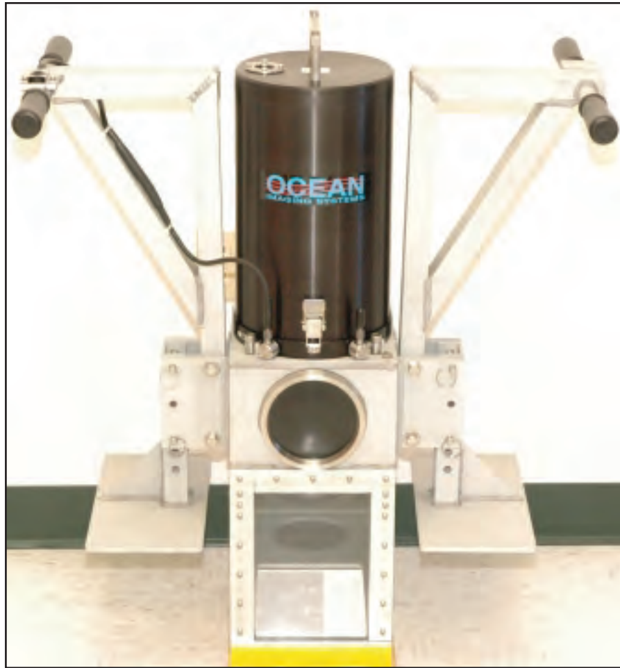
Figure 3: The hand-held SPI system used by divers for all stations that were located underneath Pier 7 at PSNS & IMF, Bremerton site.
