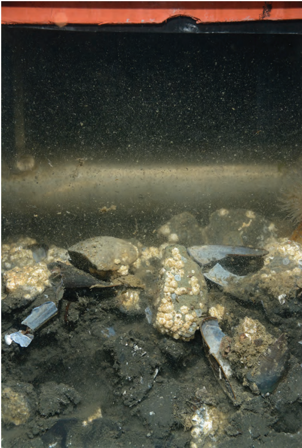
Figure 6: This profile image from Station 4-3 show an armoring of pebble and cobbles over silty very fine sand. Scale: width of profile image = 14.6 cm.
