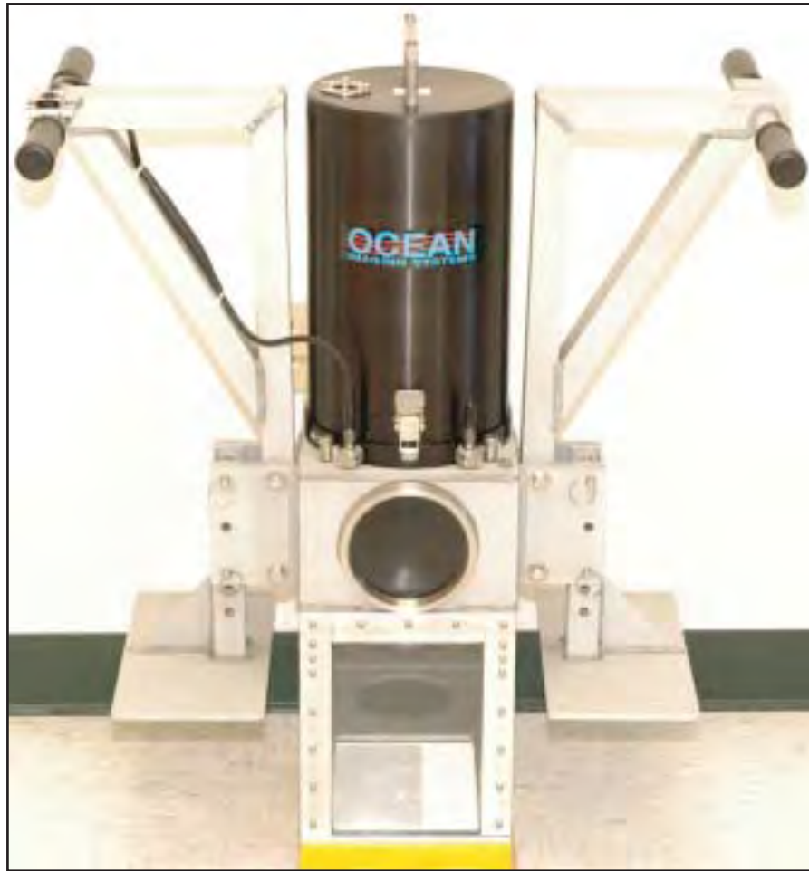
Figure 3: The hand-held SPI system used by divers for all stations that were located underneath Pier 7 in Bremerton.
