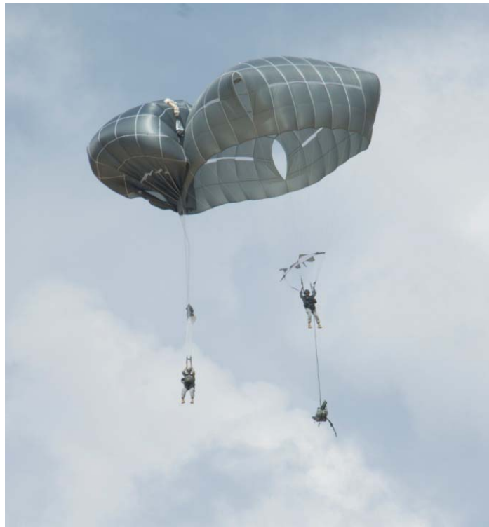
Figure 11. T-11 Corner Vent Entanglement. Source: Duncan (2016).
