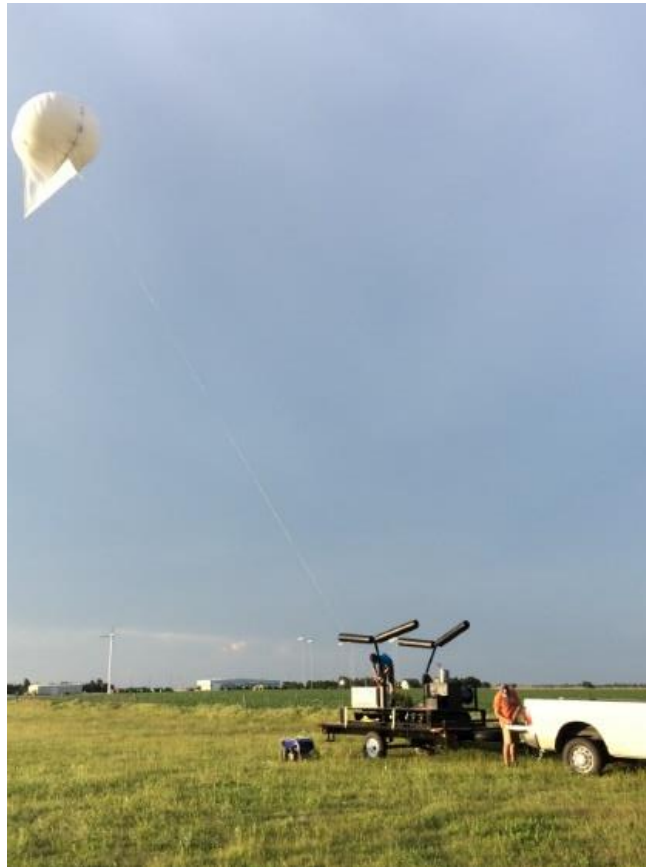
Balloon System is shown with the Helikite and the balloon mooring arms on a trailer with hydraulic winch. A generator (seen on ground) was used to power the winch and work lights during night operations.
