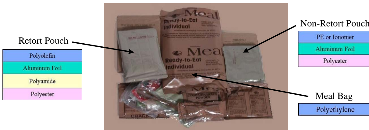
Figure 3. Current Packaging Structure of the MRE
