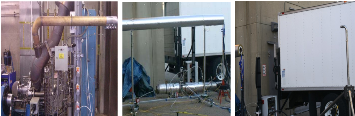
Figure 24. T63 engine with extension pipe to direct exhaust outside of the test cell for exhaust sampling with tip-diluted and gas probes at pipe exit and large gas probe at plume
