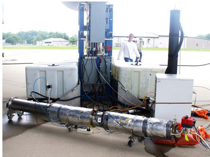
Figure 27. Dilution chamber (DC) and Condensation Dilution Probe (CDP) installed near engine during C-17 demonstration
