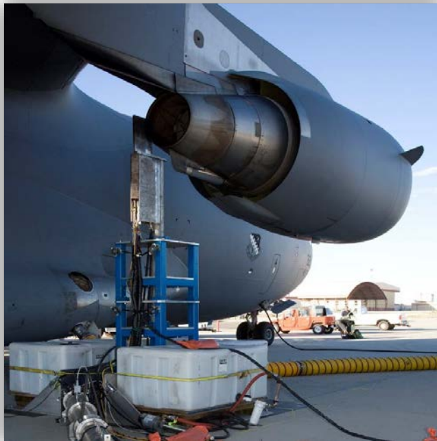
Figure 15. Demonstration platform: C-17 PW- F117 engines at WPAFB, OH
