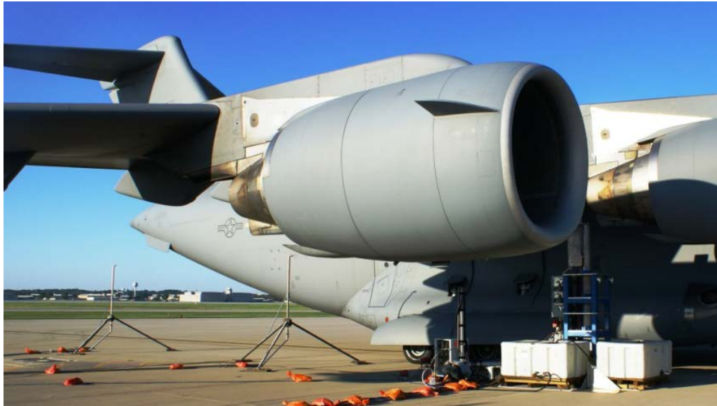
Figure 26. Emissions sampling probes at engine exit, 10m and 20 m, and probe rake for engine exit plane emission sampling
