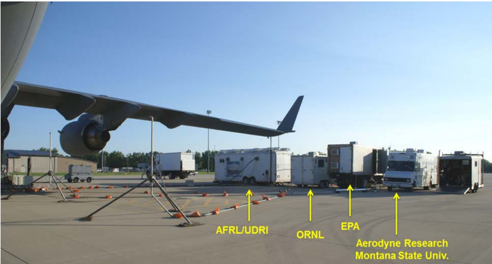
Figure 28. Emissions mobile laboratories and plume probe setup at C-17 aircraft engine emissions demonstration
