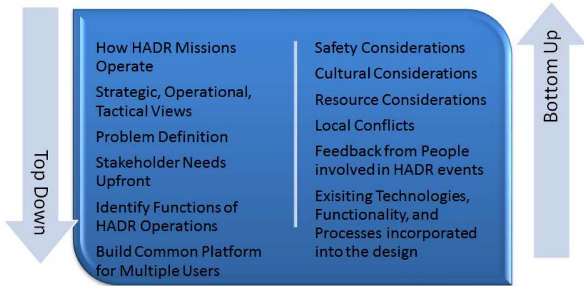
Figure 4. Top-Down / Bottom-Up Approach to Requirements Development and Architecture Design for the OMP
