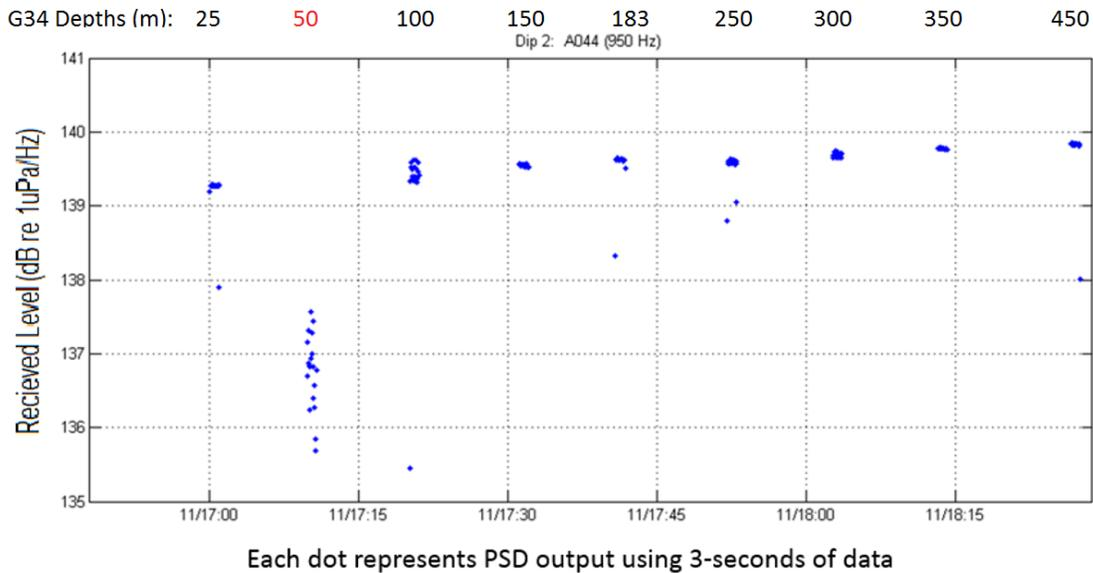
This illustrates the dispersion of received 3-second average acoustic levels measured at the source reference detector 5 meters below the projector. Notice the spread of received signals at the source level of 50 meters.
