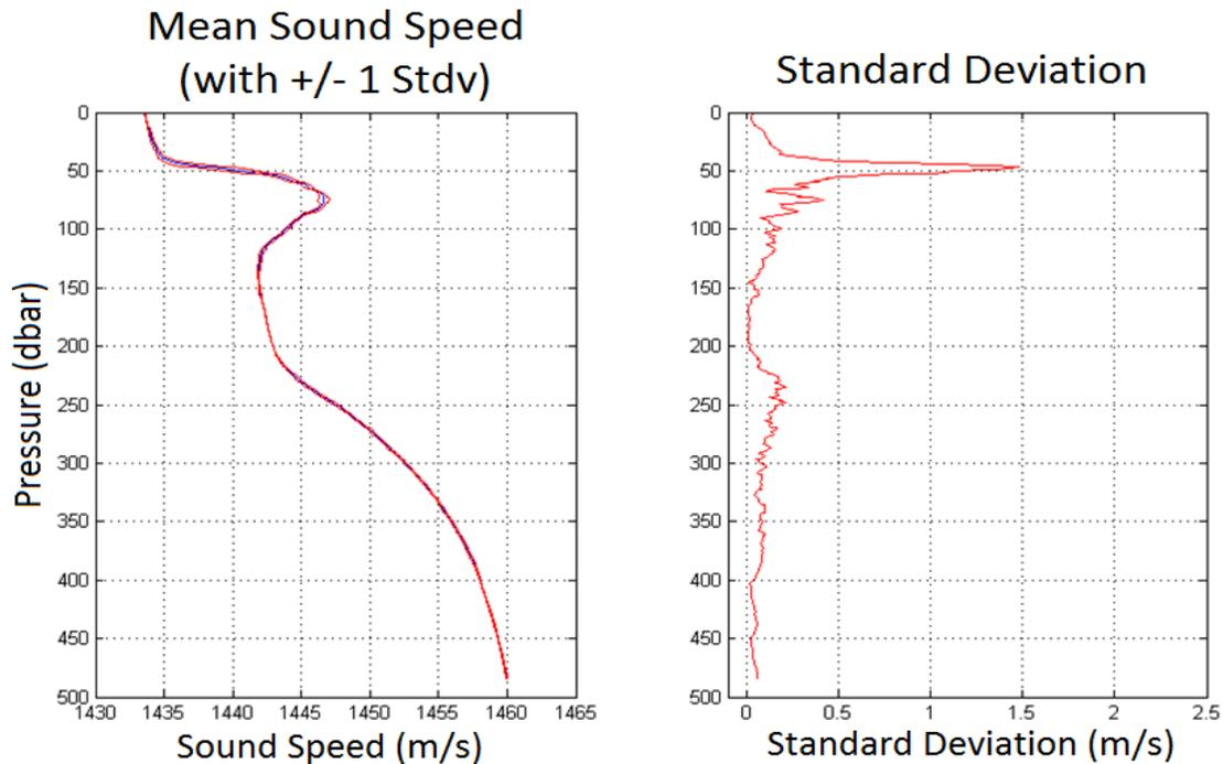
The graph on the left represents the mean sound speed profile in blue and +/- 1 standard deviation from the 7 CTD casts shown in red. The graph on the right highlights the variability identified at 50 meters.
