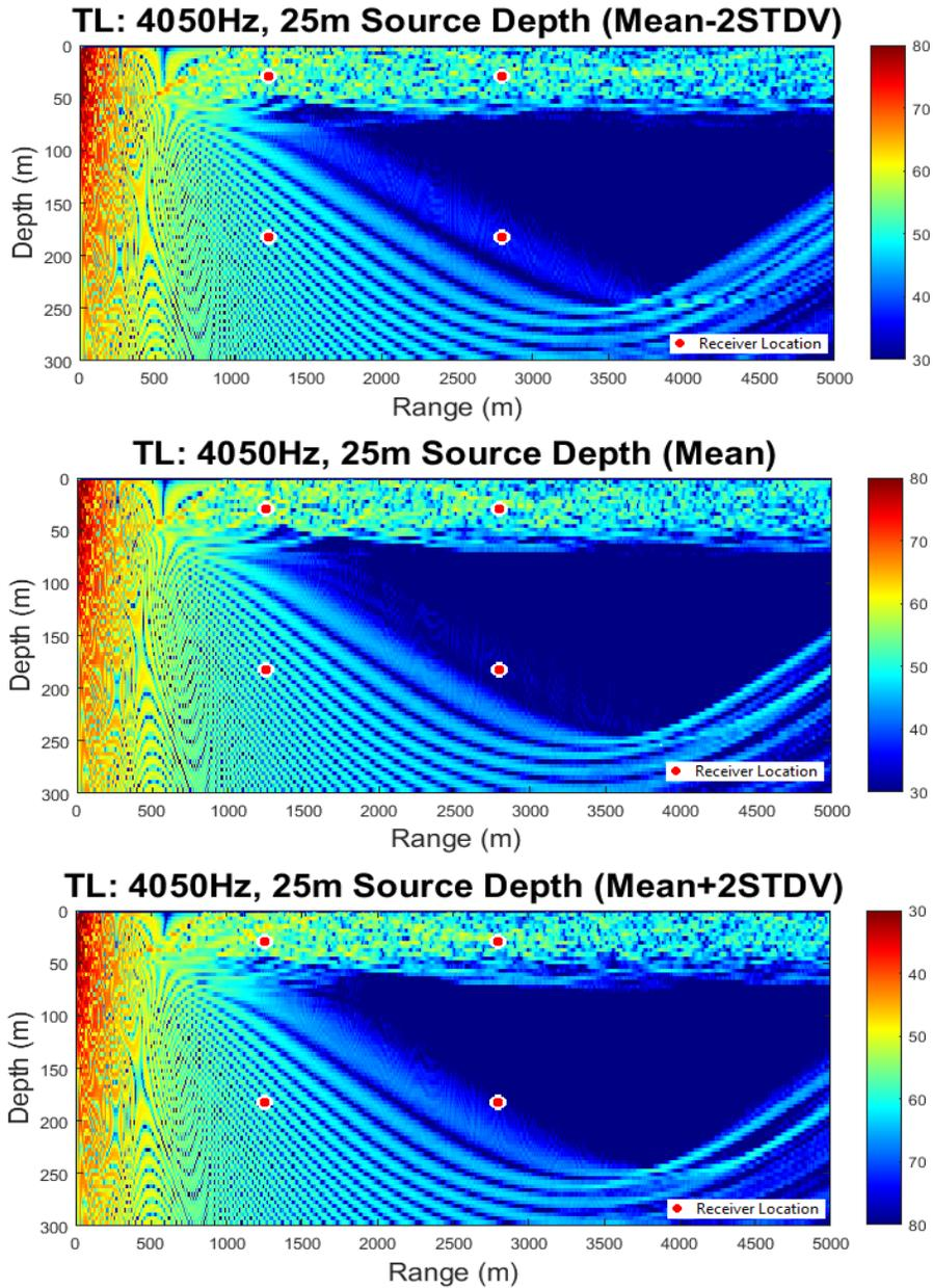
The effects of sound speed variability on transmission loss are shown by generated models of the mean and the mean  $\pm 2$  standard deviations of observed sound speed variability. The four receiver locations are shown for reference comparison.
