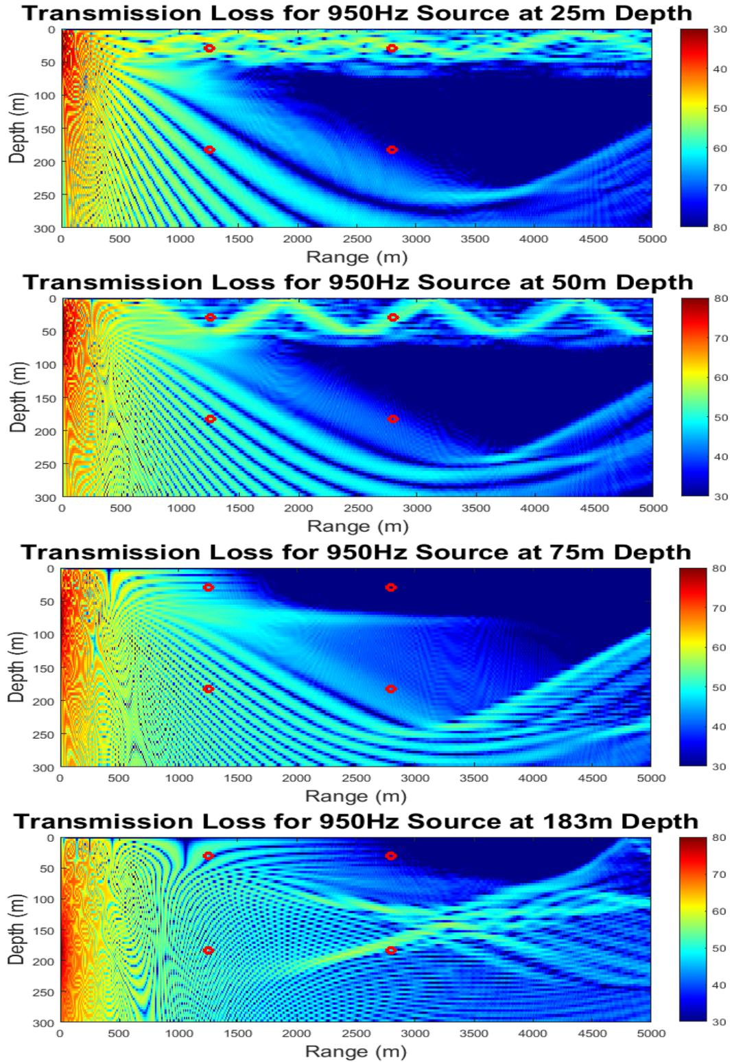
This series of models illustrates the effects of depth variability on transmission loss.
