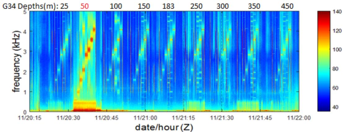
This spectrogram shows the entire range of frequencies and depths transmitted. Notice the broad frequency spectrums occurring at the 50 meter transmission depth, which may be due to turbulent flow around the receiver.
