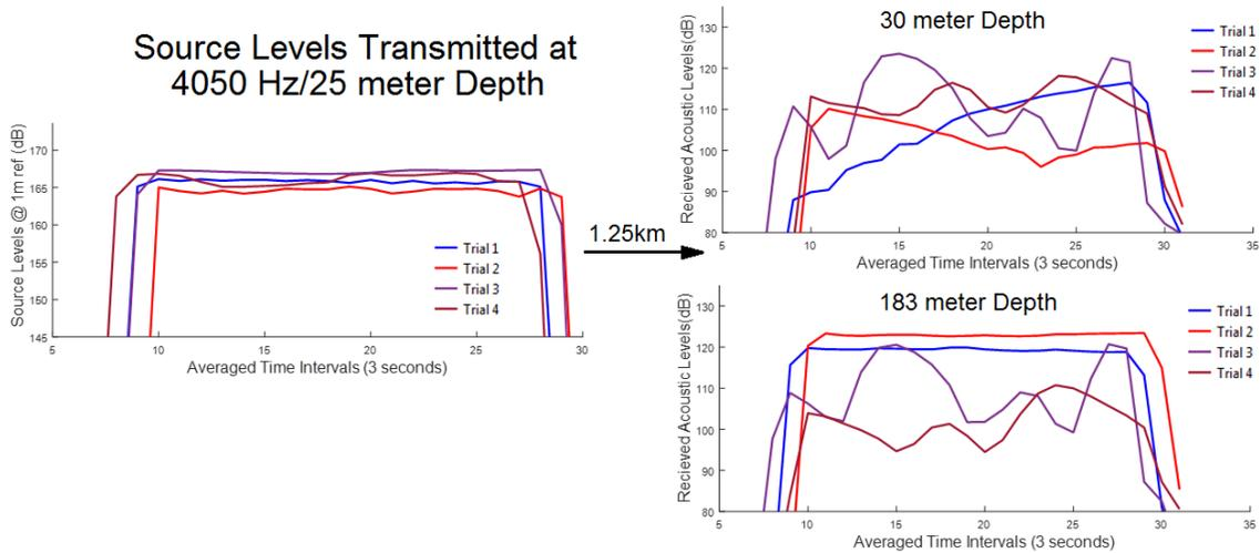
This is an extreme example of observed variability during the 57 second transmission periods. Also note the relatively steady output signal from the source, and the amount of variability between the 4 trial runs. In most cases, the monitoring hydrophone acoustic signals were represented by a flat line.
