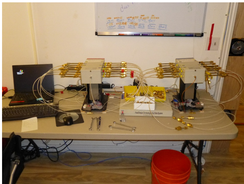
Figure 3.7. Schematic and photo of automated indoor and outdoor air sampling and concentration using multi-bed sorbent tubes.
