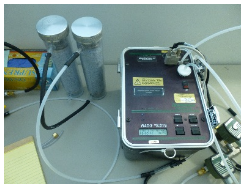
Figure 3.9. Schematic and picture of DurrIDGE RAD7 sampling assembly used for analysis of indoor air and soil gas for radon.
