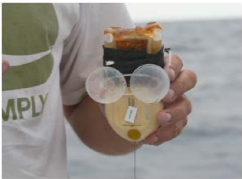
Figure 1.1 A damaged DTAG recovered from a brief deployment on a bottlenose dolphin off Cape Hatteras, North Carolina.
