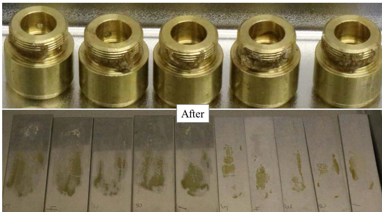
Figure 28: The visual performance of azeotrope 7 (AZ7) in the Branson 125 against marine grade grease
