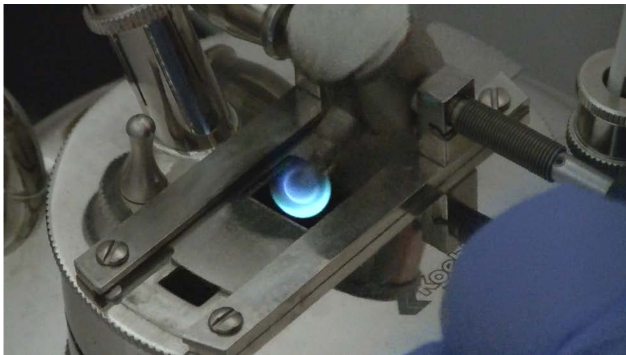
Figure 18: Photo of CBTF participating in burning below its flash point
