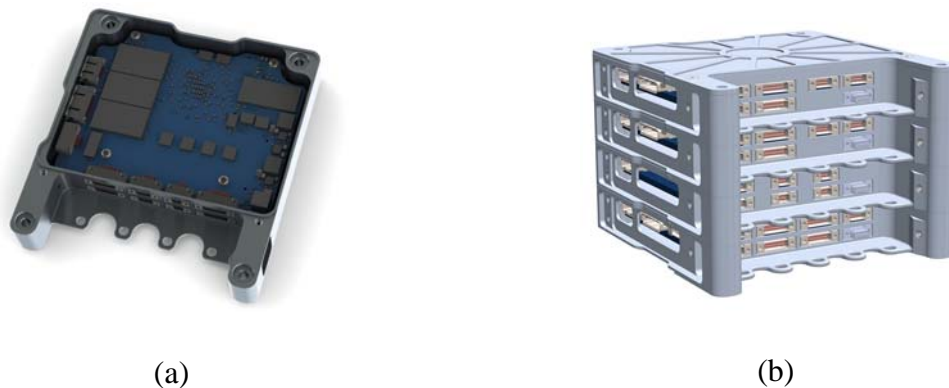
Figure 7. Data handling system (DHS). (a) Aluminum slice design. (b) Stack of four slices comprising the DHS.
