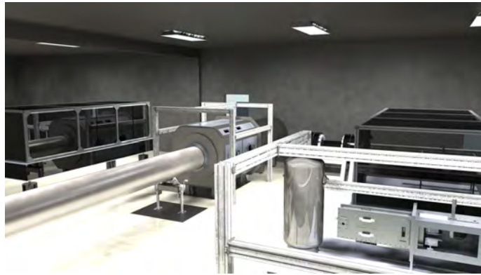
FIG. 18 The test section as it would appear at the NAL without a nozzle and with the tailpipe protruding through a wall to the outside.
