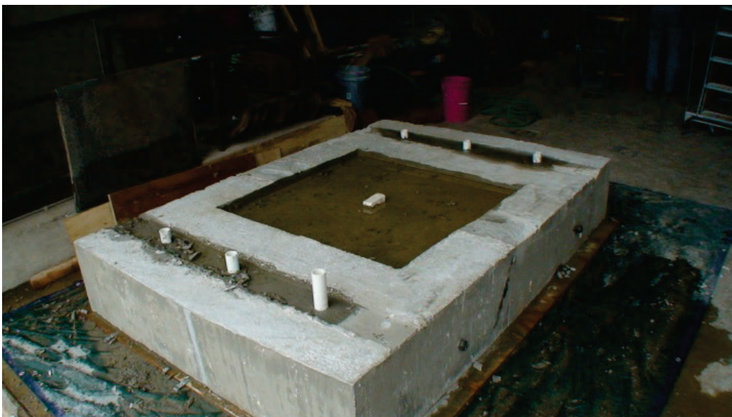
Figure 7. Concrete pad on strong-floor.
