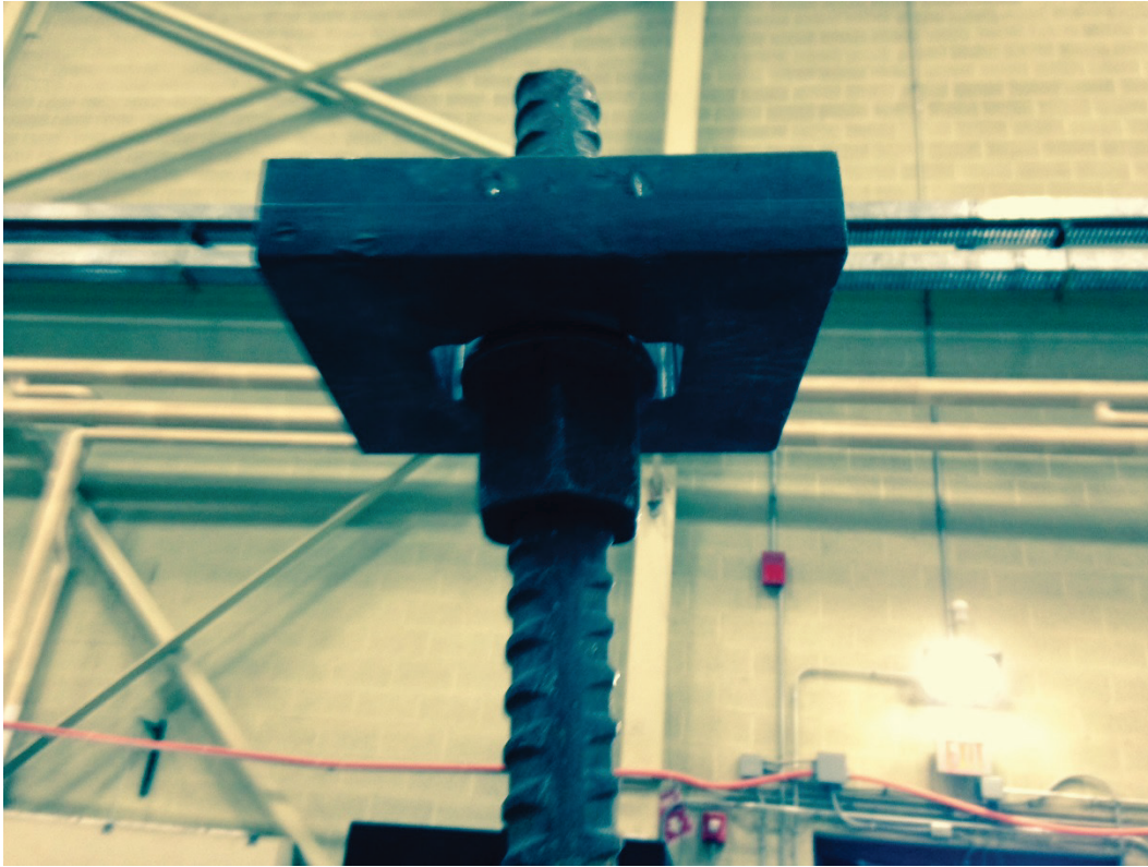
Figure 10. Photograph of special load-transfer assembly used in testing program.
