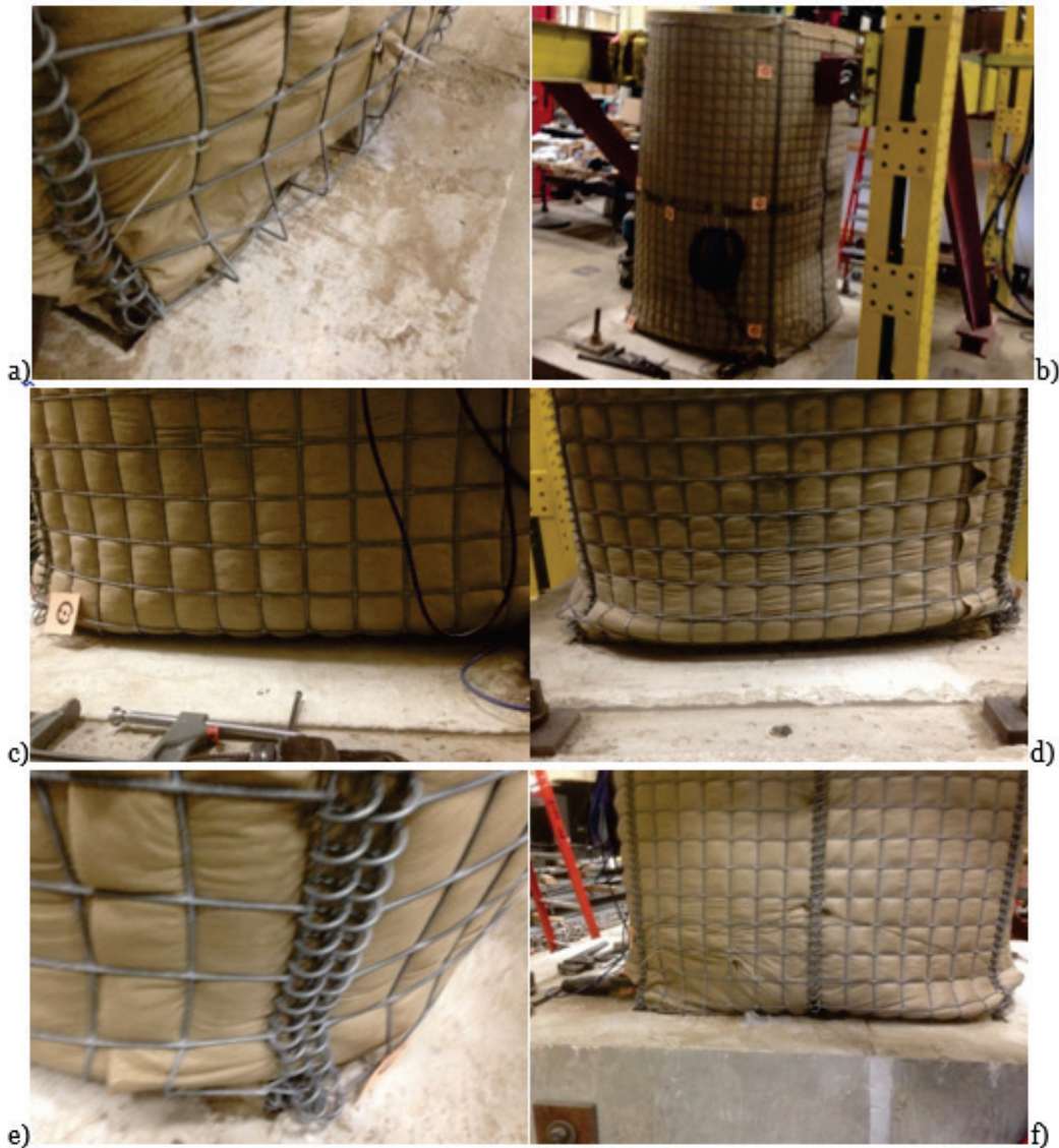
Figure 42. Photographs of failure modes seen in HESCO unit.
