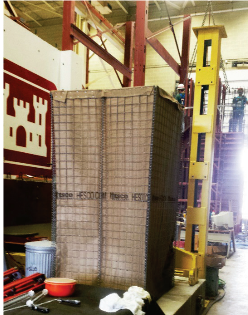
Figure 8. Exterior of unfilled HESCO bastion.
