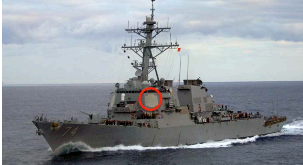
Figure 1. DDG-74 (USS McFaul) with AN/SPY-1 Radar Highlighted
