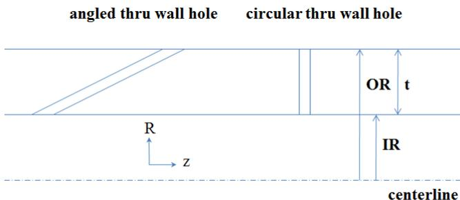
Figure 1 – Configuration of thru wall holes.
