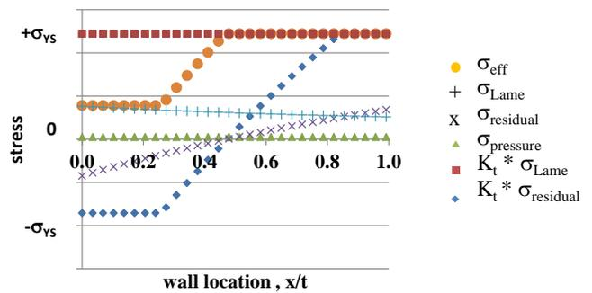
Figure 2 – Stresses present in angled thru wall hole.
