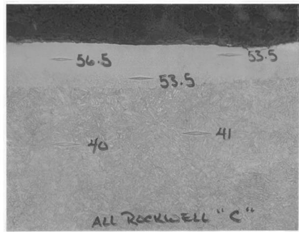
Figure 9 - White Layer and Hardness in keyway.
