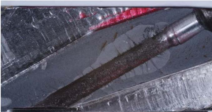
Figure 4 – Cross section of angled thru wall hole showing location of fatigue damage.
