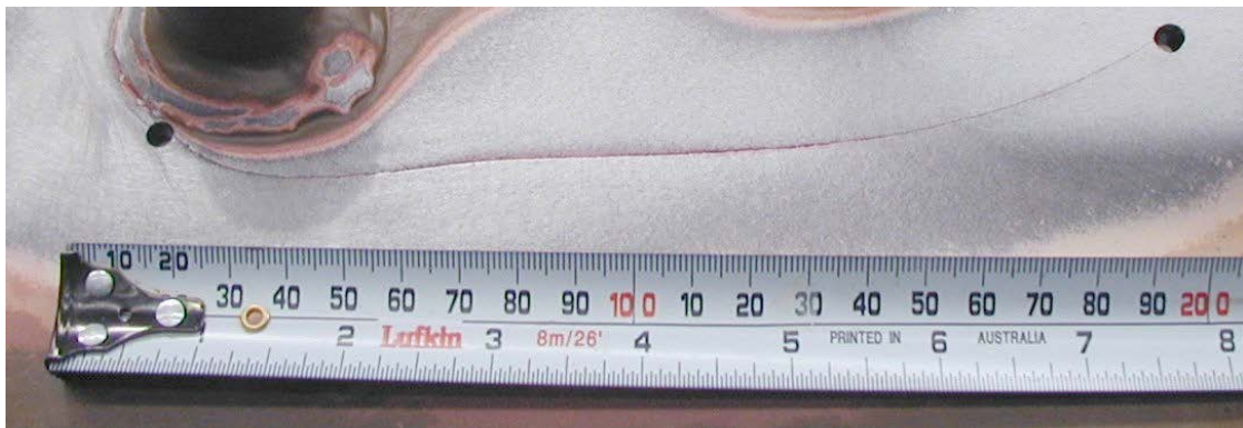
Figure 20: Structural crack in high hardness armour caused by delayed cracking (after [55]). This crack is over 200 mm in length.
