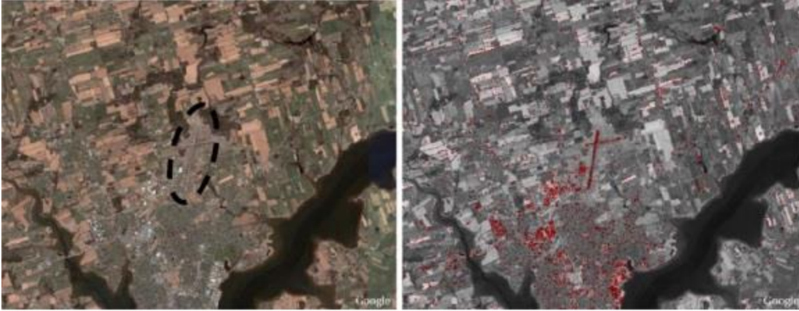
Figure 1. Original Image (Left) with the Runway Enclosed in Dashed Lines. Detected Runway Blocks are Shown in Red (Right)
