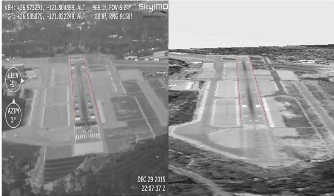
Figure 39. Line Projection Mismatch in Real Implementation (Left) and Match in Simulation (Right) for Monterey Regional Airport
