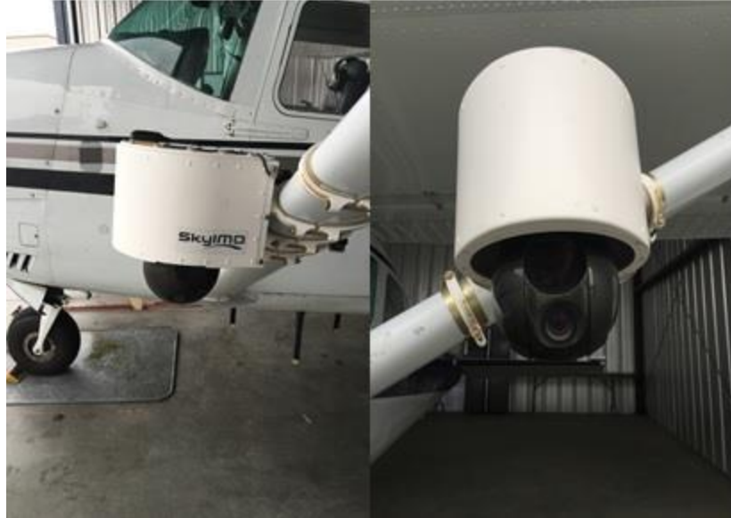
Figure 31. Camera TASE200 Mounted on the Cessna 206 Airplane
