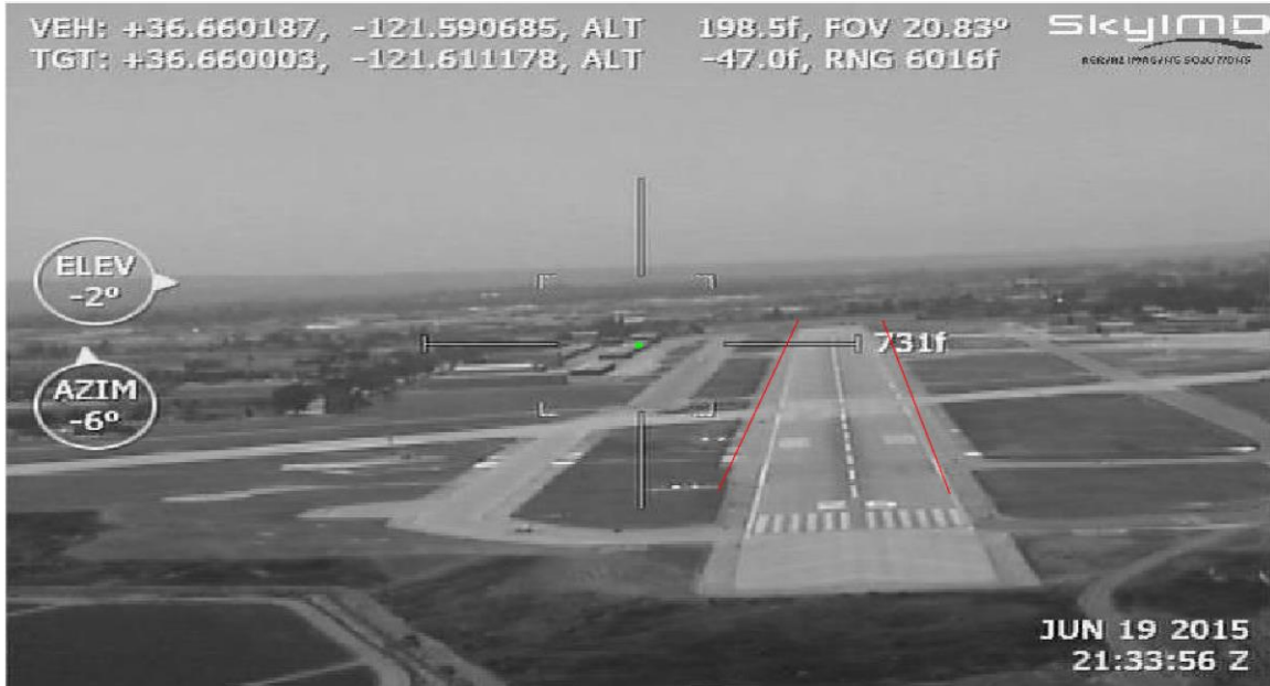
Figure 36. Runway Detected on the Real Camera View from Salinas Municipal Airport
