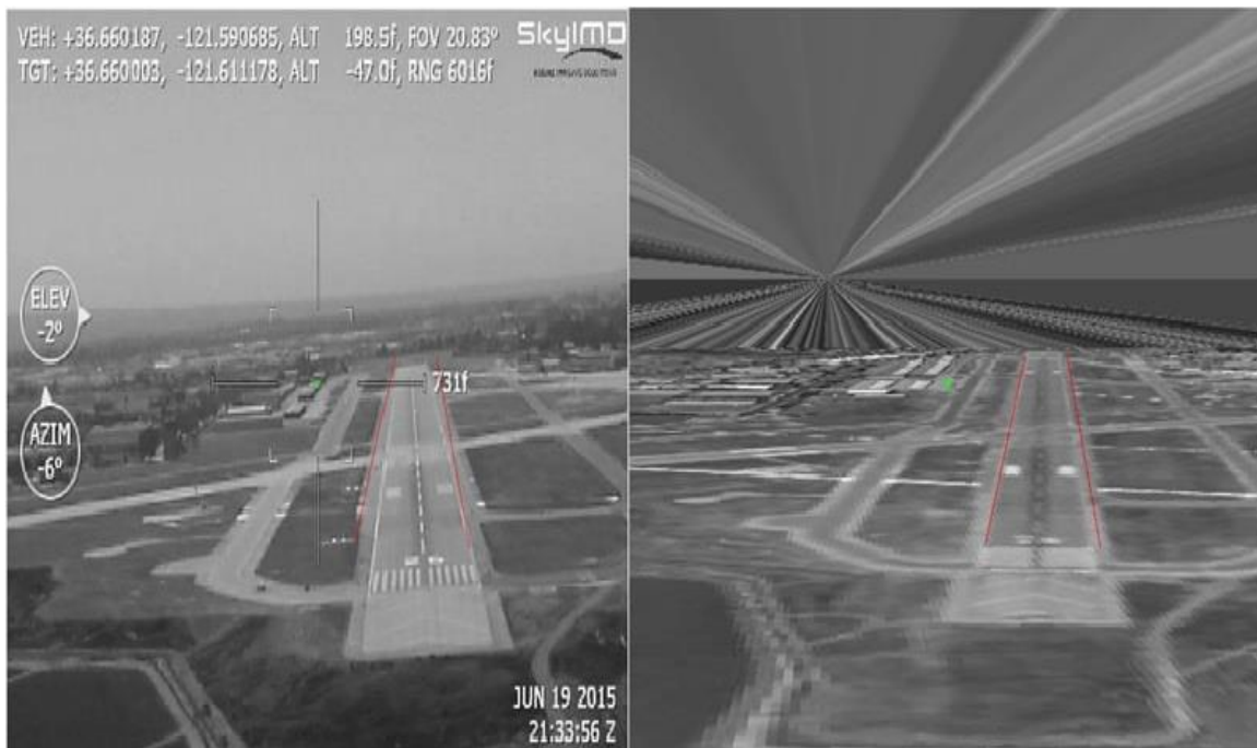
Figure 38. Line Projection Mismatch in Real Implementation (Left) and Match in Simulation (Right) for Salinas Municipal Airport
