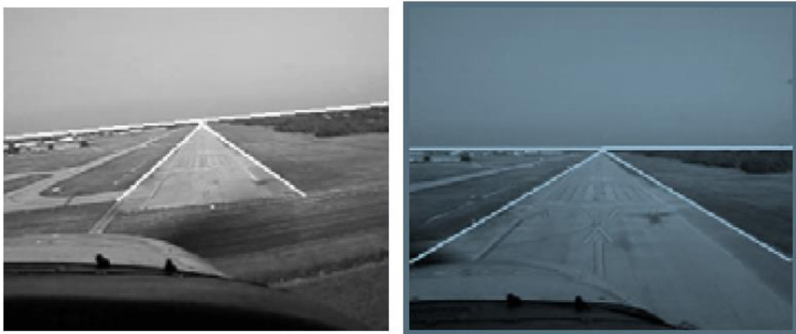
Figure 3. Detection Results for Runway and Horizon, Highlighted with a White Line
