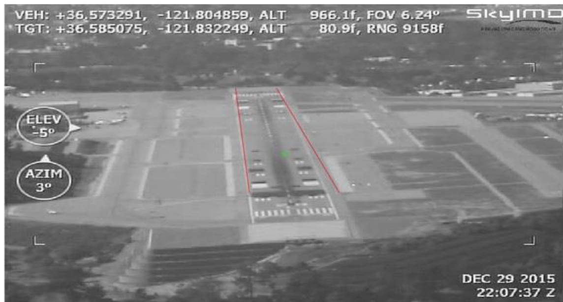
Figure 37. Runway Detected on the Real Camera View from Monterey Regional Airport
