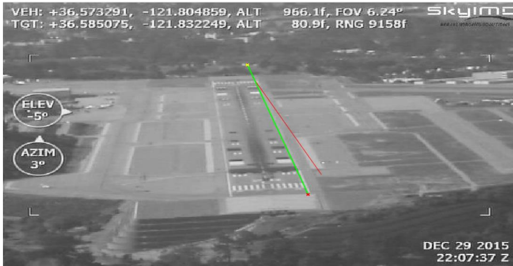
Figure 44. Mismatch in Right Projected Line and Correction by Hough Transform in Monterey Regional Airport
