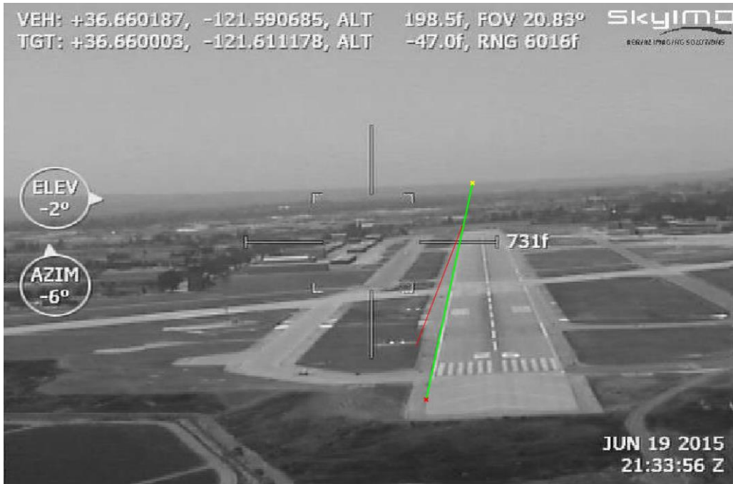
Figure 41. Left Edge (Green) of Salinas Municipal Runway Detected by the Hough Transform Closer to the Projected Left Line (Red)
