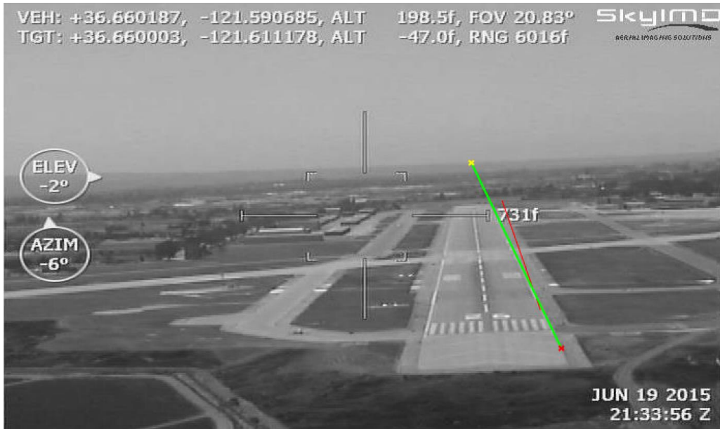
Figure 42. Right Edge (Green) of Salinas Municipal Runway Detected by the Hough Transform Closer to the Projected Right Line (Red)
