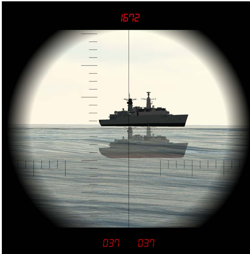
Figure 14. Outside View with Stadimeter Applied.
