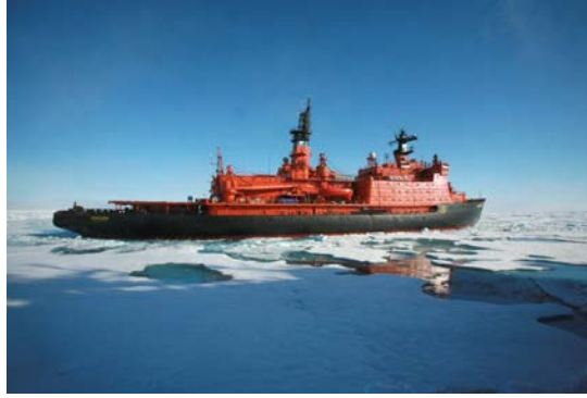
Figure 6. Wall-Sided Hull (Rossiya, Russian Icebreaker). Source: [13].
