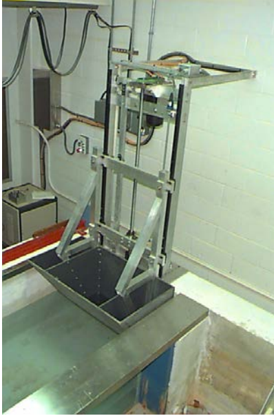
Figure 55. U.S. Naval Academy Plunger Wave Maker. Source: [30].
