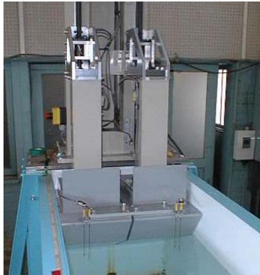
Figure 51. Plunger Wave Generator. Source: [28].
