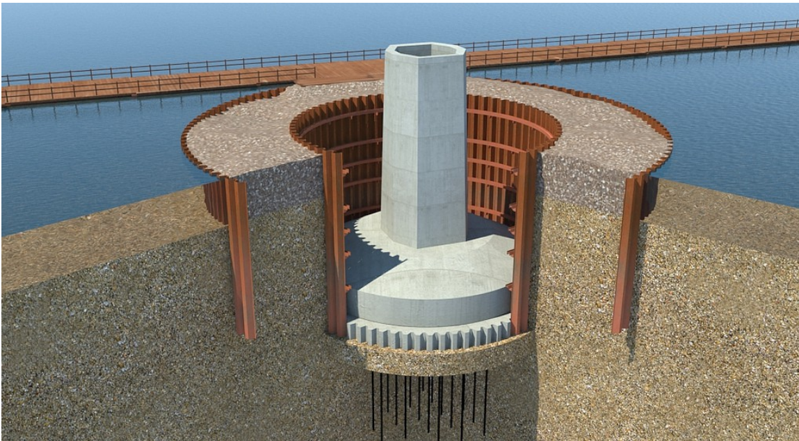
Figure 11. Cofferdam with sheet metal walls and gravel filling between the walls. Source: [14].
