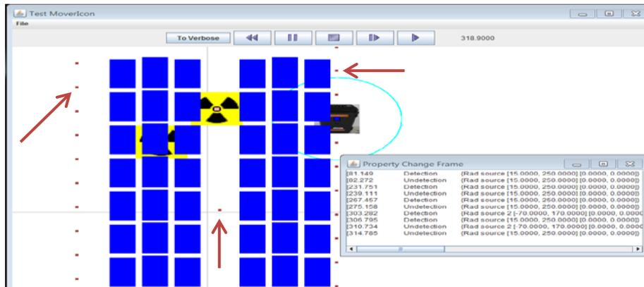
There are numerous waypoints as highlighted by the red arrows, each of which will be a stopping point for the Polaris. Source: Screen capture from Simkit.
