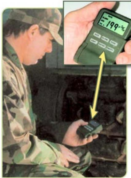
The radiac device displayed is a Canberra product that detects radiation in a given area. A device of this size and design makes it easy for users to navigate as well as operate. Source: “RGU-100” (n.d.).
