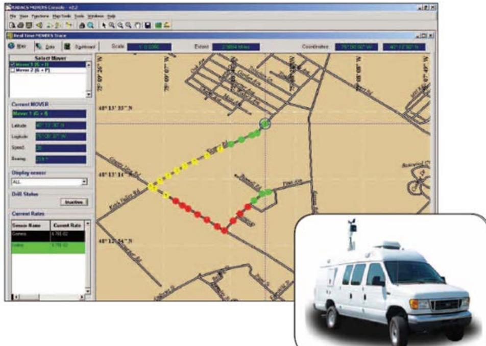
Mobile Vehicle based Emergency Radiation Monitoring System (MOVERS), located inside the van, detects radiation and tracks the location of those measurements on software provided to the user. Source: "Movers," (n.d.).
