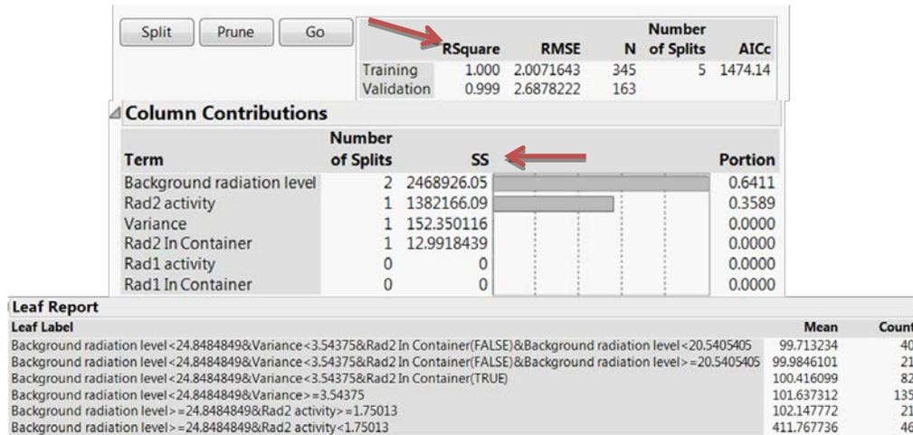
The R-square value has increased when doing modeling via partition tree instead of using a fit model. The column contribution highlights the summary of squares, marked SS, and states which factors had the higher proportion. Source: JMP Screen Shot.
