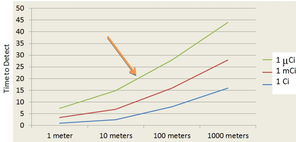
The continuous line of each measurement from DTRA's deterministic model of the Polaris 2.1 indicates there is a point at which there will always be a detection while in range.
