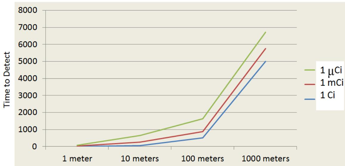
Adapted from DTRA's deterministic model is a fictitious representation of the Polaris 2.1 detecting a heavy shielded radiation source.
