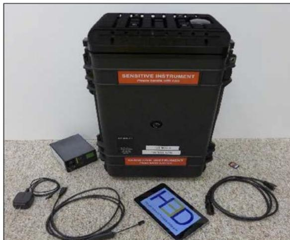
The Polaris 2.1 gamma ray imaging device detects, identifies, and locates radiation in a given area. With the Polaris are cables, battery, and a tablet to be used by the operator. Source: H3D et al. (2015, p. 6).
