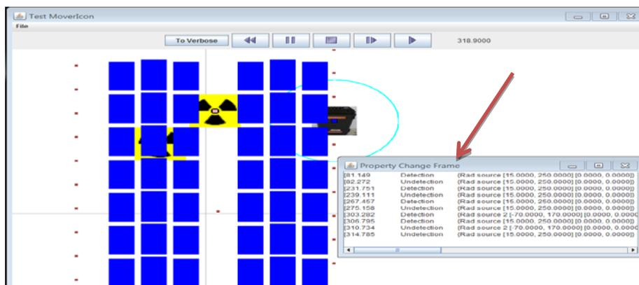
The arrows points to the property change frame which can be prompted to display every detection and undetection. Source: Screen capture from Simkit.
