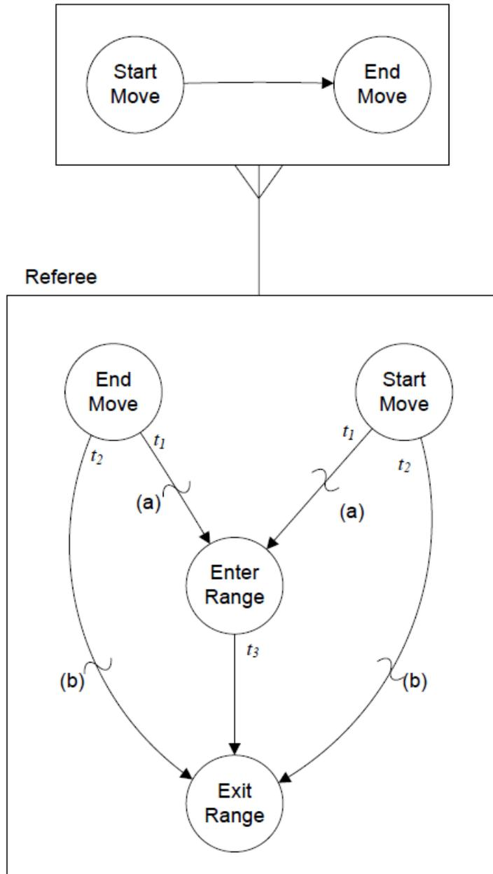
The referee listens to the start and stops of the mover and determines whether or not the Polaris has entered or exited the range of the radiation source. The (a) and (b) annotate a Boolean for entering and exiting range, and for this DES that Boolean was either greater or less than a set distance. Source: Buss & Sanchez (2005, p. 997).
