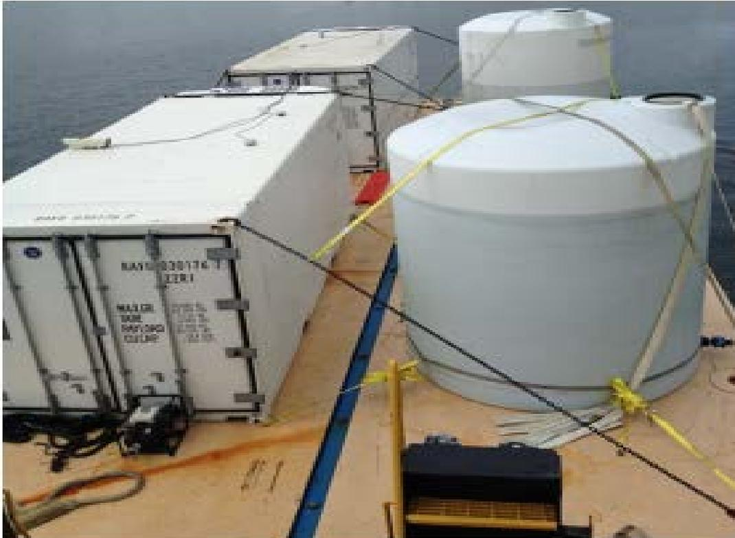
The SuperMISTI detects radiation and gives the user an image overlaid a real image of the direction it is sensing. This figure displays the SuperMISTI inside the two large white rectangular containers with two water tanks alongside that act as a counter balance for the motion of the water. Source: Hutcheson et al. (2012, p. 362).
