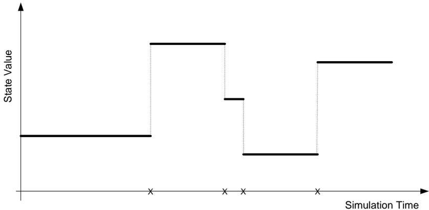
The values of the state variable change instantly from one state to another during the simulation, thus piecewise. As such, a modeler always knows the state of an entity at any given time during the simulation. Source: Buss (2011, p. 5).
