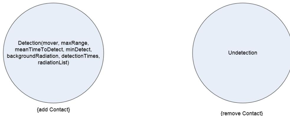
The Polaris Constant Rate Sensor is an extension of the Basic Sensor, taking into account the Polaris Mover, mean time to detect, minimum detection level, background radiation level, an array of detection times and an array of radiation sources. Source: Polaris Constant Rate Sensor Source Code.
