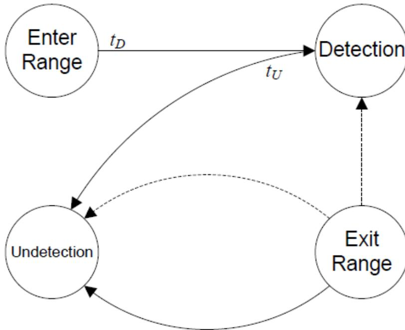
The mediator event graph displays calculation time between entering the Polaris range and actual detection of the radiation source. The Polaris DES time for undetection ( $t_U$ ) is always zero whereas the time for detection ( $t_D$ ) is dependent on many factors incorporated into this model such as radiation strength and background radiation. The Source: Buss & Sanchez (2005, p. 998).
