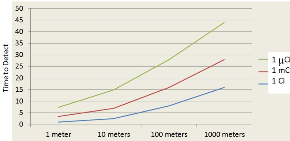
Adapted from DTRA's deterministic model is fictitious representation of the Polaris 2.1 detecting a lightly shielded radiation source.
