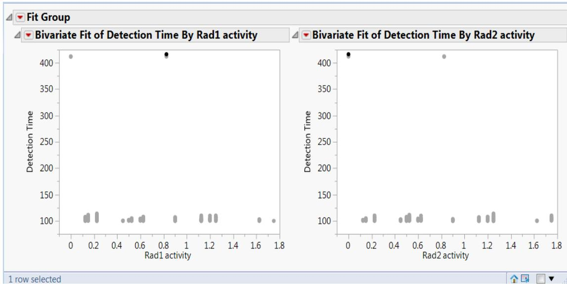
The image above has two data points that are highlighted in black. Each of those marks a time when the detection times were remarkably high, nearly four times the mean. As seen above, when the radiation activity level is at 0.001 for either radiation source 1 or radiation source 2, the corresponding detection times were above 400. Source: JMP screen shot; data from Simkit.
