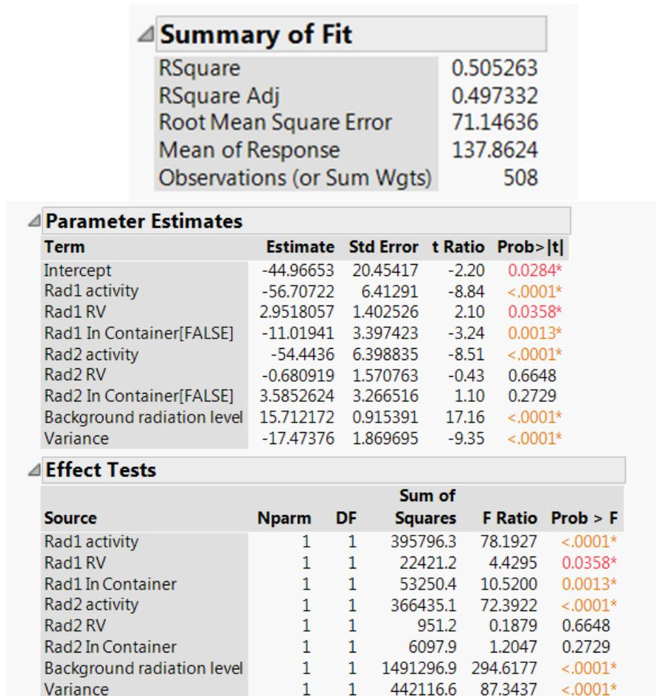
JMP output from data collected from discrete event simulation model shows the different significance each variable. Although the numbers highlighted in orange and red are significant, the R-Square value is relatively low at 0.505. Source: Screen capture from JMP; data pulled from Simkit.
