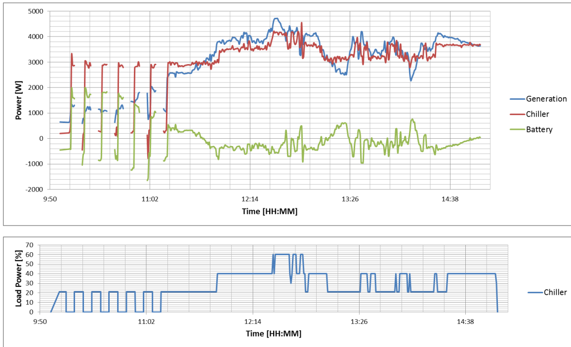
Figure 29. Control Data Running Chiller
