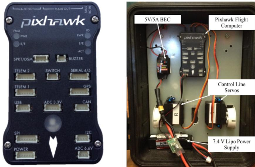
Figure 16. Pixhawk Flight Computer and Installation in Prototype Snowflake ADS
