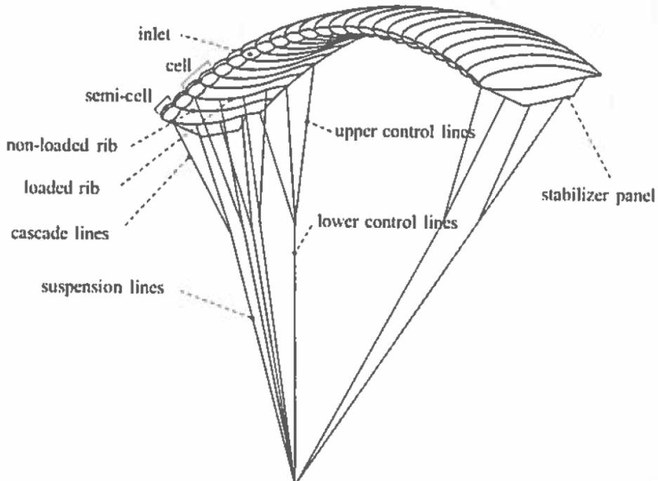
Figure 1. Basic Ram-Air Parachute. Source: Lingard (2015).
