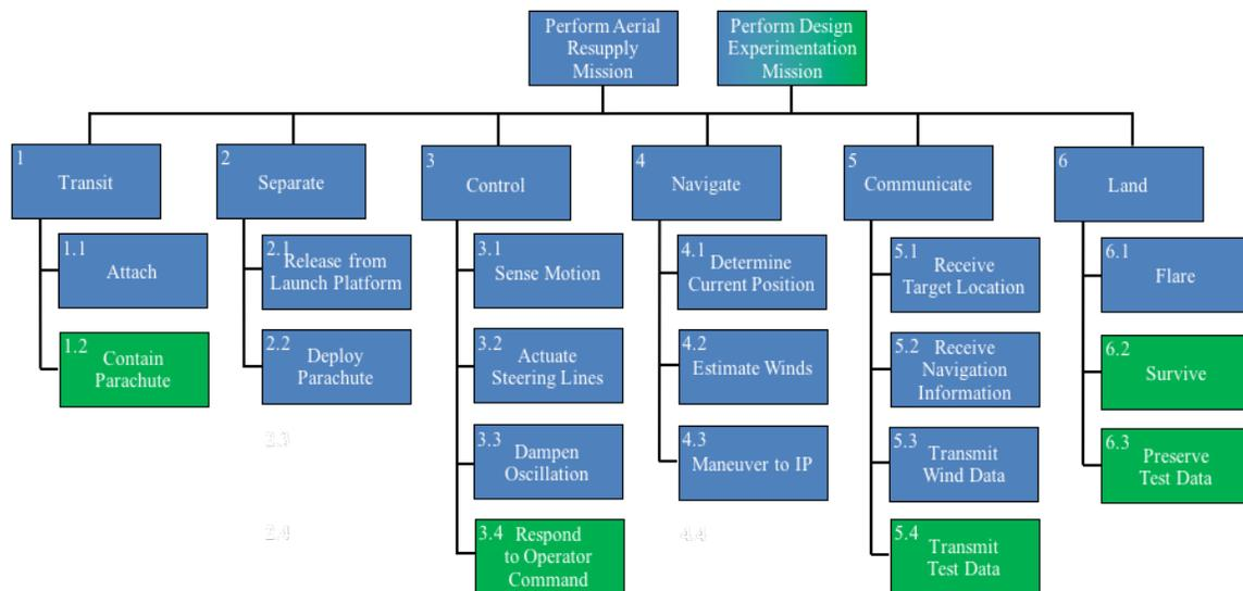
Figure 13. Functional Hierarchy of Two PADS Missions
