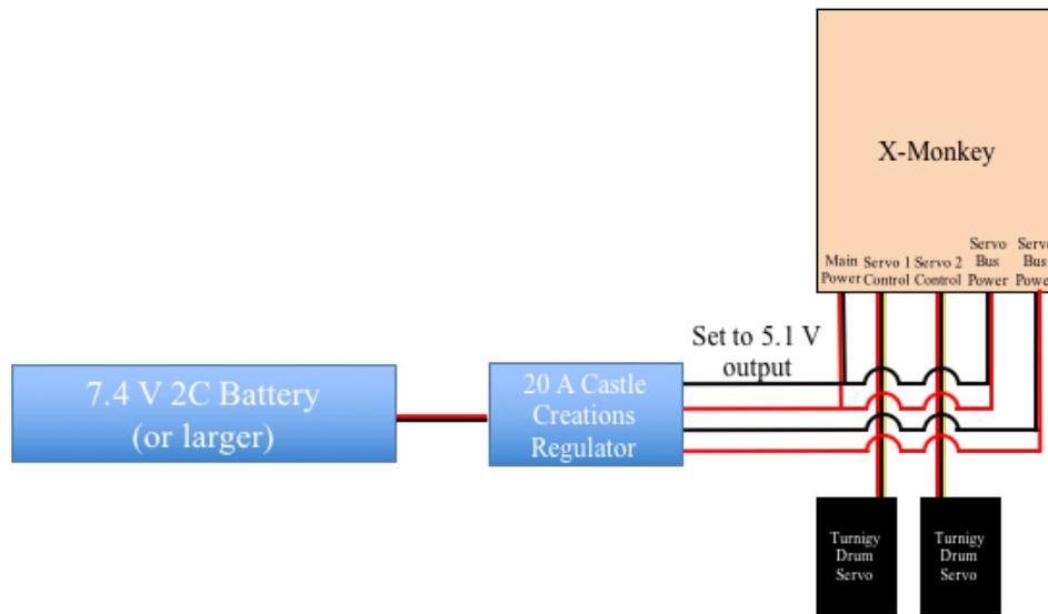
Figure 19. Electrical Power Distribution for Snowflake ADS
