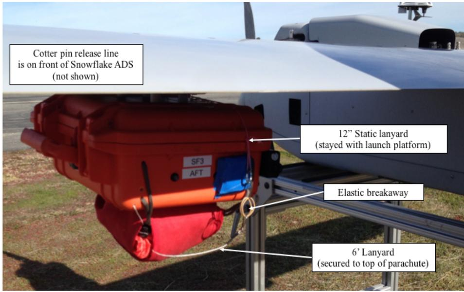
Figure 27. Installed Double Static Line
