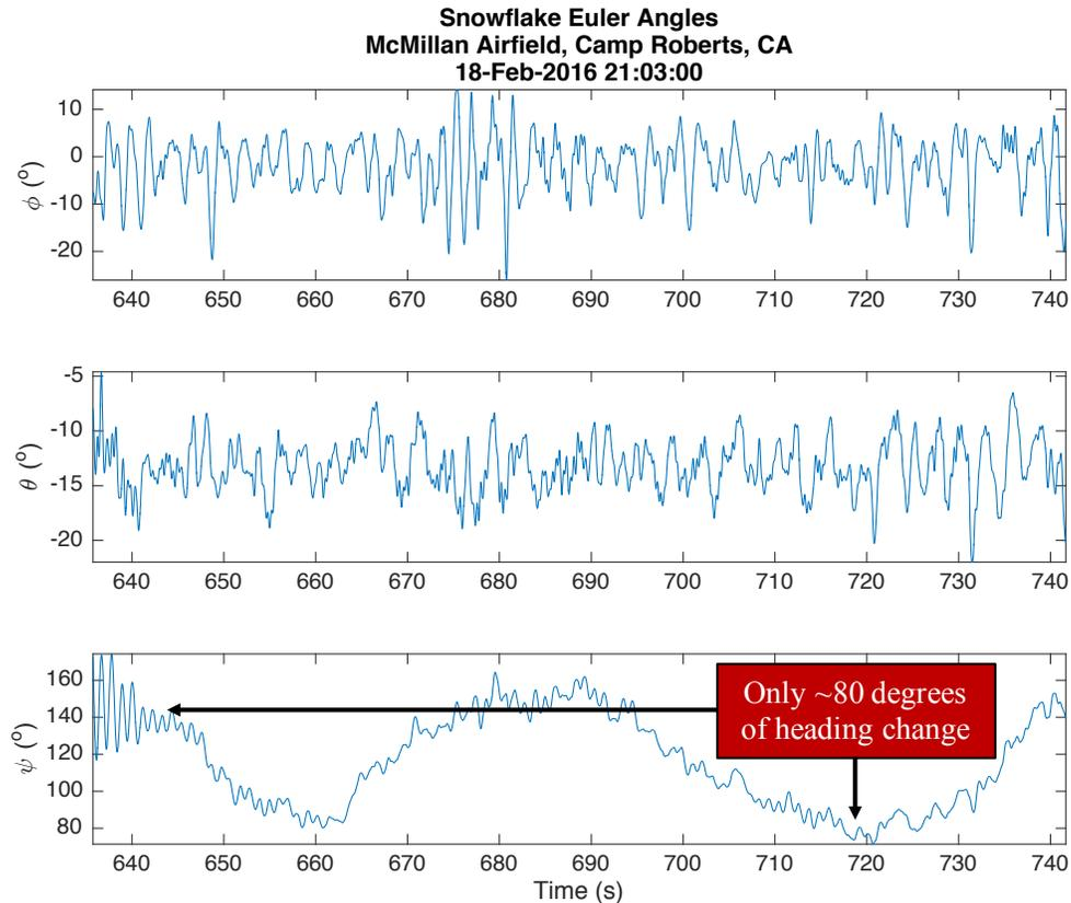
Figure 41. Flight Test Results: Snowflake Euler Angles
