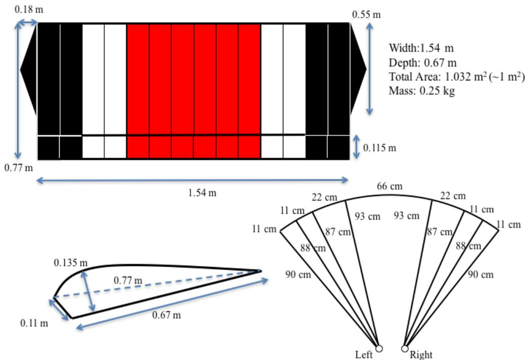
Figure 21. Overhead, Side and Control Line Specifications for 1 m<sup>2</sup> Rectangular Ram-Air Parachute
