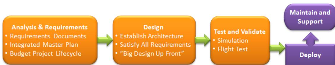
Figure 7. PD-PLDC “Waterfall” Methodology. Source: Barber, Montague and Barelo (2011).
