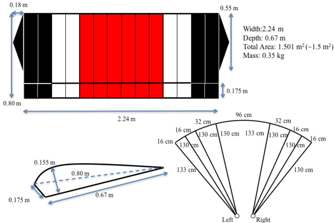
Figure 22. Overhead, Side and Control Line Specifications for 1.5 m<sup>2</sup> Rectangular Ram-Air Parachute
