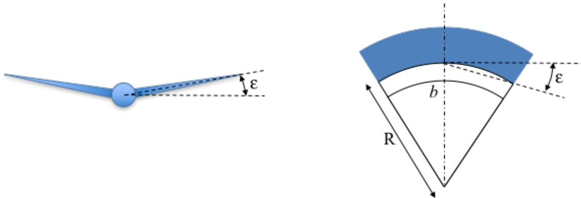
Figure 2. Contrast of Conventional Wing Dihedral and Ram-Air Wing Anhedral. Adapted from Lingard (2015).
