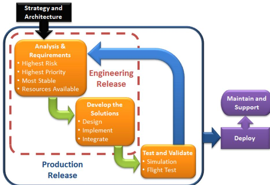
Figure 8. Airborne Systems Agile Methodology for U.S. DOD Programs. Source: Barber, Montague and Barello (2011).
