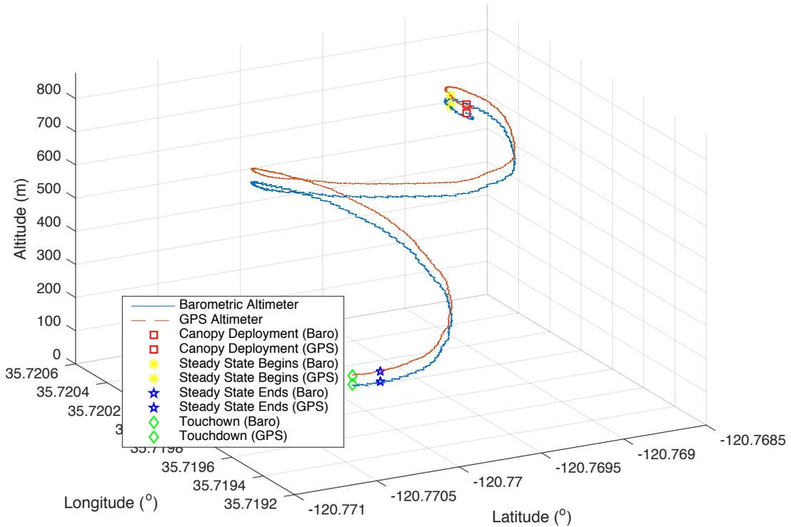
Figure 38. Flight Test Results: Three-Dimensional View
