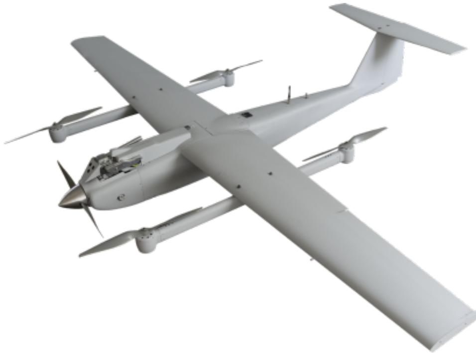
Figure 15. Arcturus VTOL Version (JUMP 20). Source: Arcturus UAV (2015b).
