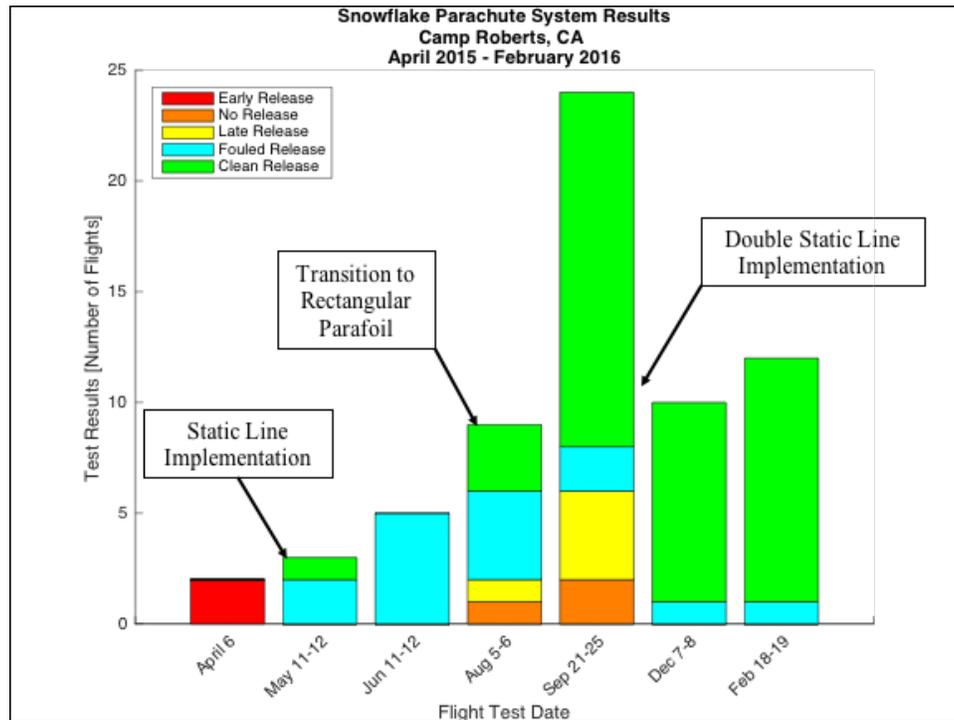
Figure 30. Failure Analysis of Snowflake Parachute Deployment Methods
