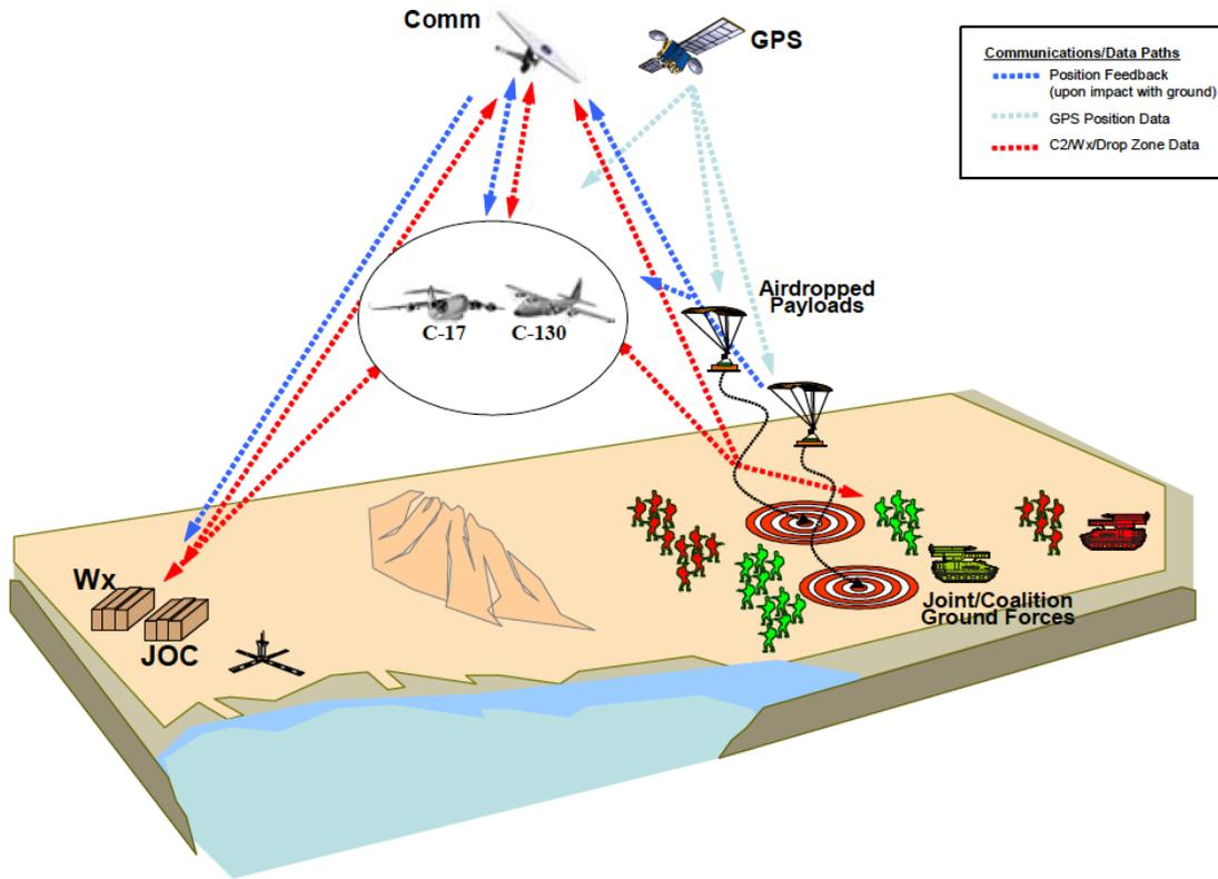
Figure 12. Precision Airdrop Combat Delivery Missions (OV-1). Source: Benney et al. (2005b).
