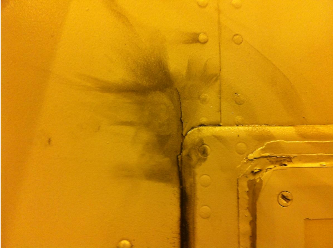
Figure 3. Fuselage Skin Crack on F/A-18D requiring ISR.
