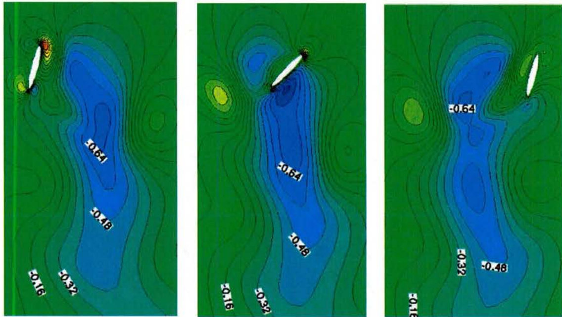
Figure 2.5-5. Illustration of the jet flow feature which develops in the path of the airfoil. Velocity contours are displayed (red: positive, blue: negative) with select percentages of the maximum translational velocity marked. In Figure 4 these snapshots would correspond to points 2 , 6, and 10 respectively.
