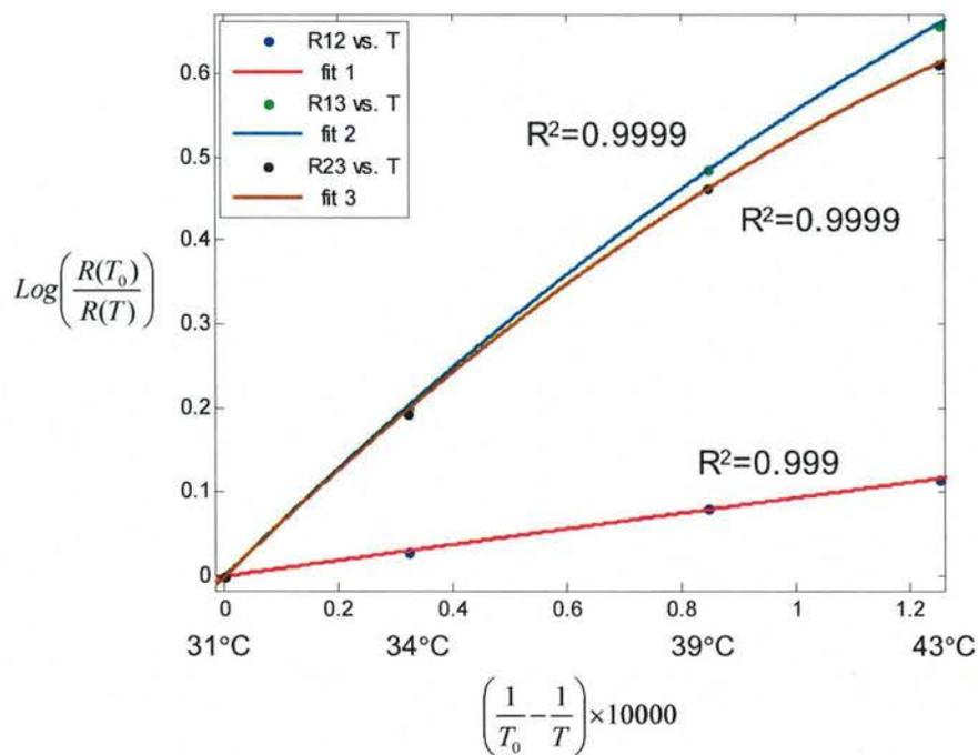
Fig. 7 The temperature calibration using laser-induced fluorescence technique.  $T_0$  is the reference temperature. The intensity ratio R12, 625 nm $\uparrow$  and 600 nm; R13, 625 nm $\uparrow$  and 568 nm and R23, 600 nm and 568 nm.
