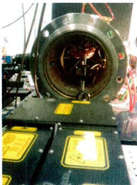
Figure 3. High-pressure chamber equipped with counterflow burners and a state of the art DPIV system.
