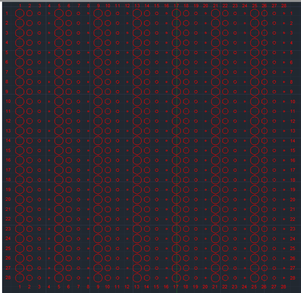
Fig. 1 Computer-aided design drawing of an example square symmetric device layout pattern: 28 \times 28 devices, alternating in device size from 300, 200, 100, and 50 microns throughout each row
