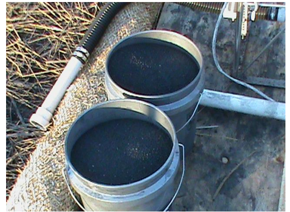
Figure 7-1 Pelletized Carbon as SediMite™
