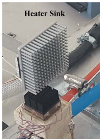
Figure 7. Heater with Sink at \theta=90^\circ
