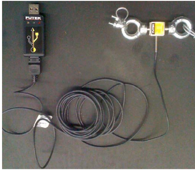
Figure 11. FUTEK Strain Gauge Used for Thrust Model Development
