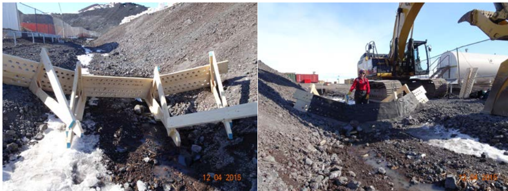
Figure 10. Prototype unanchored wooden weir tested along one of the channels. The left photo is the downstream side of the weir. The right photo is the upstream side of the weir.
