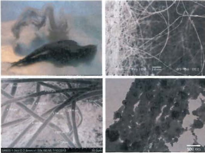
Figure 2. Electrospun control polystyrene fibers (white) and PS fibers loaded with 11 wt% n-Al/PFPE (dark grey) (top left). SEM images of: pure PS fibers (top right), and PS fibers electrospun with 6 wt% n-Al/PFPE (lower left). TEM image of PS fibers electrospun with 17 wt% n-Al/PFPE (lower right).
