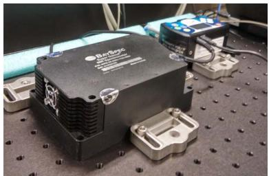
This is the Bayspec near-infrared (NIR) spectrophotometer that collects the nanocrystal emission with a fiber. This grant also supported the purchase of other equipment like a Newport solar simulator, a 488 nm Coherent OBIS laser, a Stanford Research Systems Lock-In Amplifier 830m, a Picoharp 300 and an InGaAs camera for NIR time-resolved experiments, various optical accessories from Newport and Thorlabs, as well as work by Physical Plants to install electrical and water cables.
