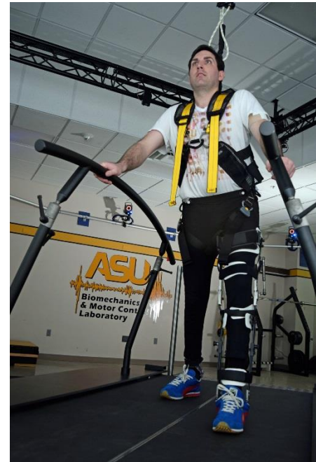
Figure 3 - Data collection for a student driven project to develop a stance control orthosis for a person with spinal cord injury.
