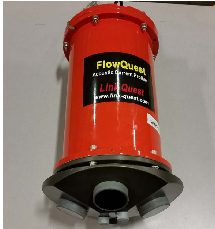
Figure C-1. A LinkQuest FlowQuest 1000 ADCP. The piezoelectric oscillators can be seen on the sloped surfaces at the bottom of the image.
