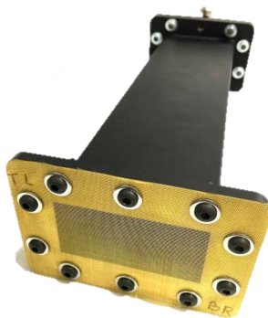
Fig. 4: Custom waveguide with brass mesh window for visualization.
