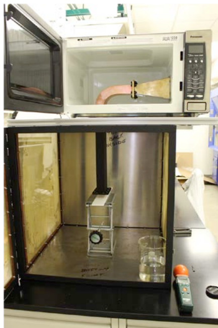
Fig. 9: Custom microwave/Faraday cage setup for large-scale microwave exposure.
