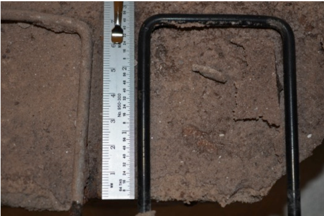
Figure 37. Destructive inspection of the interior of a galvanized (left) and vitreous coated (right) pintle after 18 months of exposure at Duck, NC.
