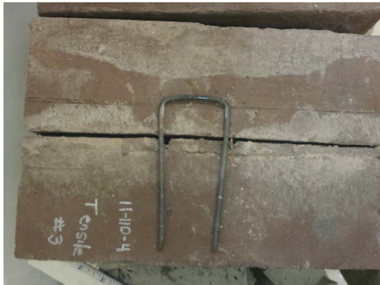
Photo 3 – Mortar Bond Failure on One Side
