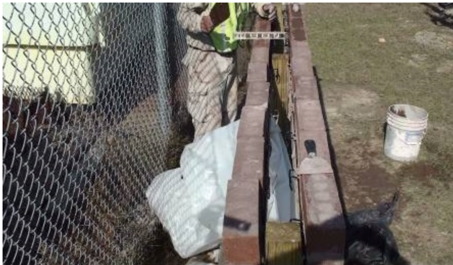
Figure 18. Fort Stewart coupon test rack.
