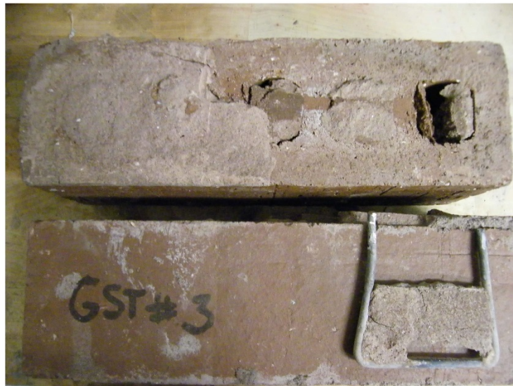
Photo 7 – Mode of Failure – GST #3
