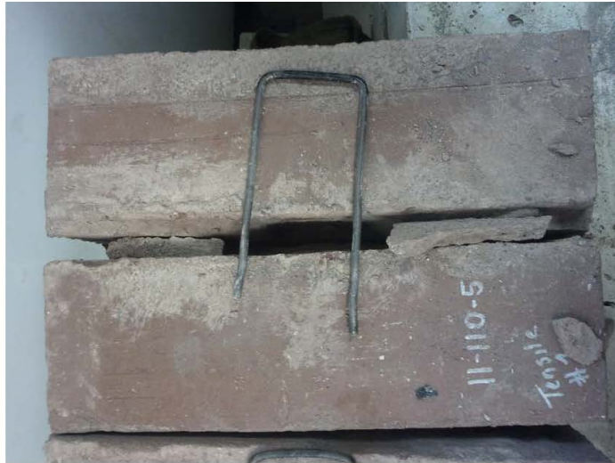
Photo 3 – Mortar Bond Failure on One Side
