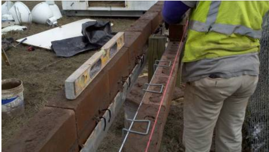
Figure 16. Production of ASTM E754 coupons.
