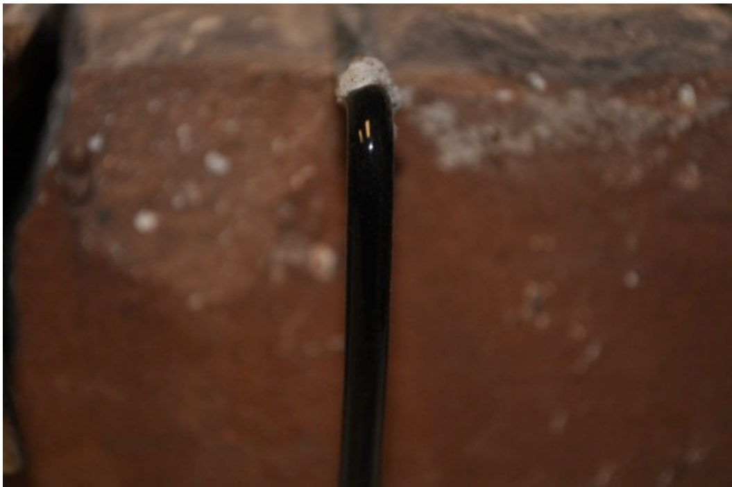
Figure 31. Inspection of the exterior part of the vitreous coated pintle after 18 months of exposure at Fort Stewart, GA.
