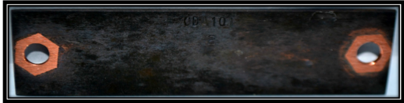
Figure 9: CDA101 Sample prior to Corrosion Removal
