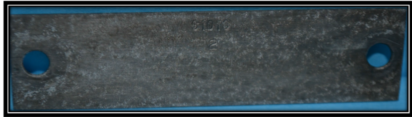
Figure 8: C1010 after Corrosion Removal
