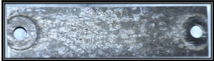
Figure 5: AL7075 T6 Sample prior to Corrosion Removal
