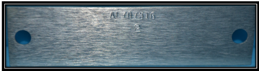
Figure 6: AL7075 T6 after Corrosion Removal
