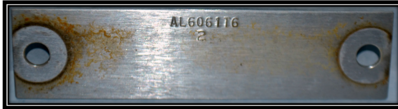
Figure 1: AL6061 T6 Sample prior to Corrosion Removal
