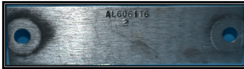
Figure 2: AL6061 T6 after Corrosion Removal
