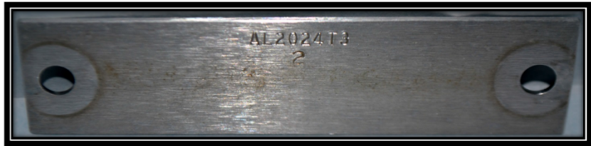
Figure 3: AL2024 T3 Sample prior to Corrosion Removal
