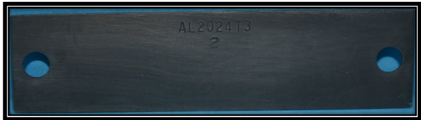
Figure 4: AL2024 T3 after Corrosion Removal
