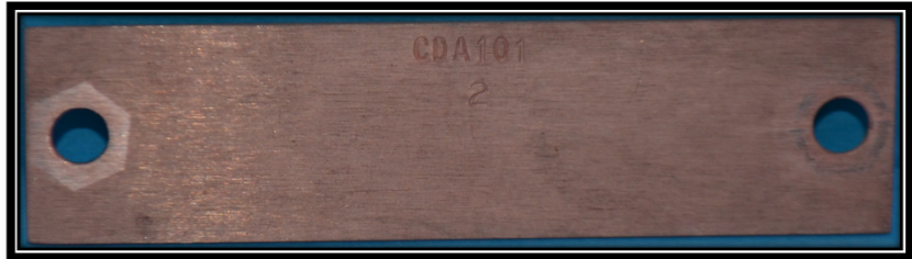
Figure 10: CDA101 after Corrosion Removal
