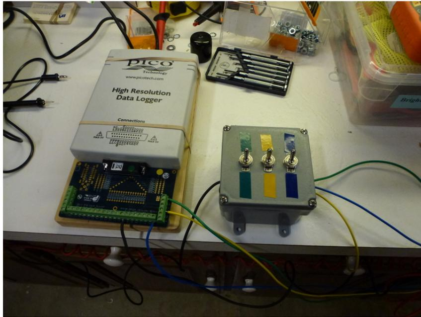
Figure A5. Commercial recording voltage meter connected to switch-box.
