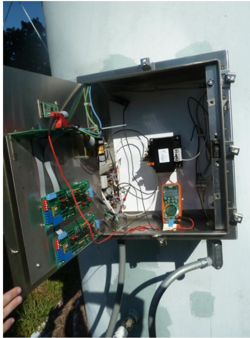
Figure C3. Prototype data logger being used for polarization-decay measurements for tank shown in Figure C1.
