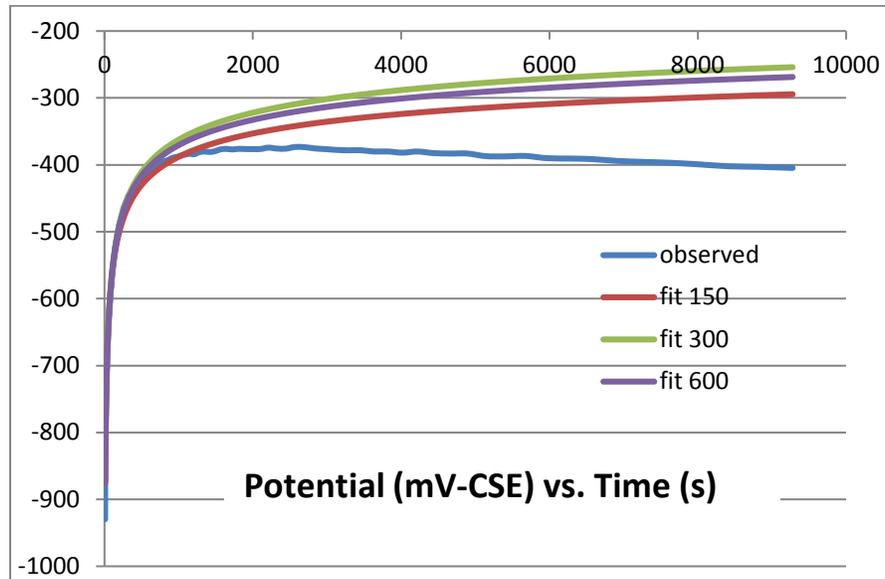
Figure 5. The first 500 seconds of data and curve-fit trend lines from Figure 4.
