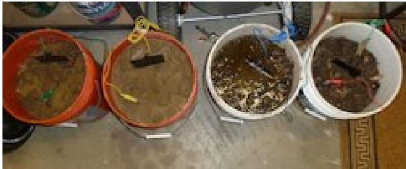
A third set of triplicate panels was used for outdoor laboratory testing, buried in native soil outside the laboratory of Bushman and Associates in Medina, OH (see Figures A8 and A9). ICCP was applied to these outdoor specimens.
